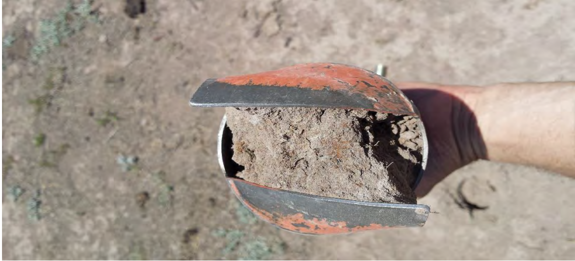
Figure 11. Iron Concentrations and Depleted Soils within the Pan Wetlands with the Soft Plinthic Soil Horizon
