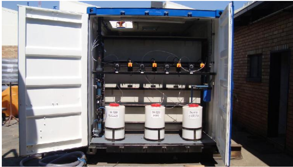
20 m 3 /h Veolia Water Botswana – Shakawe – Containerized PWTP – Botswana
