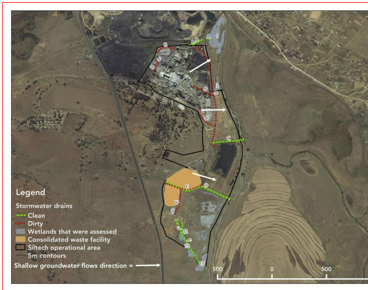
Figure 5-2: The movement of surface storm water and ground water at the site in relation to the wetlands on site (Source: Ikhwane Wetland Science, 2020)
