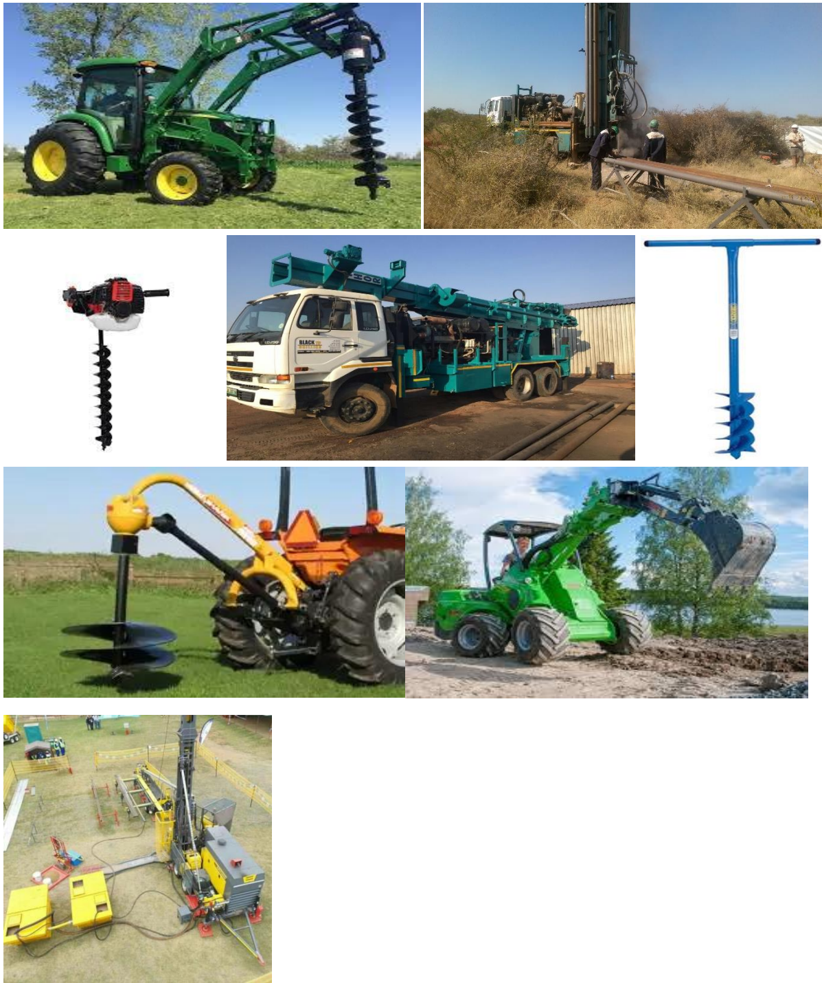
Figure 4 : Typical example of air flush drilling machine with the compressor mounted on the truck, hand auger drill and tractor mounted auger drill (all will possibly be used in sand and clay exploration).
