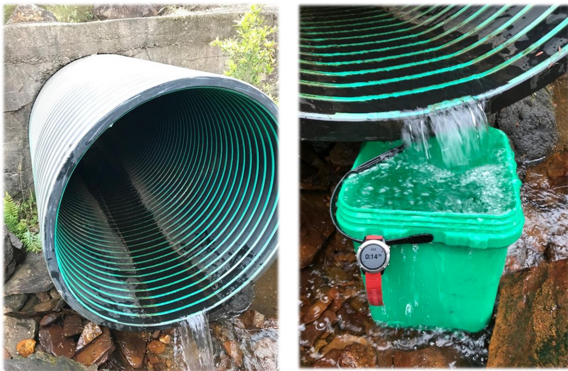
Figure 3. Measured flow (15 July 2022) at the weir in the unnamed stream directly downstream of the local catchment.
