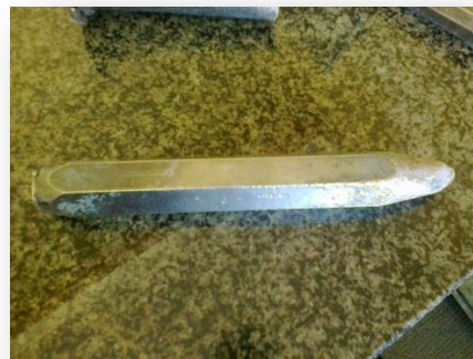
An example of a pointed chisel used to plane the granite blocks to give it a smoother look.
