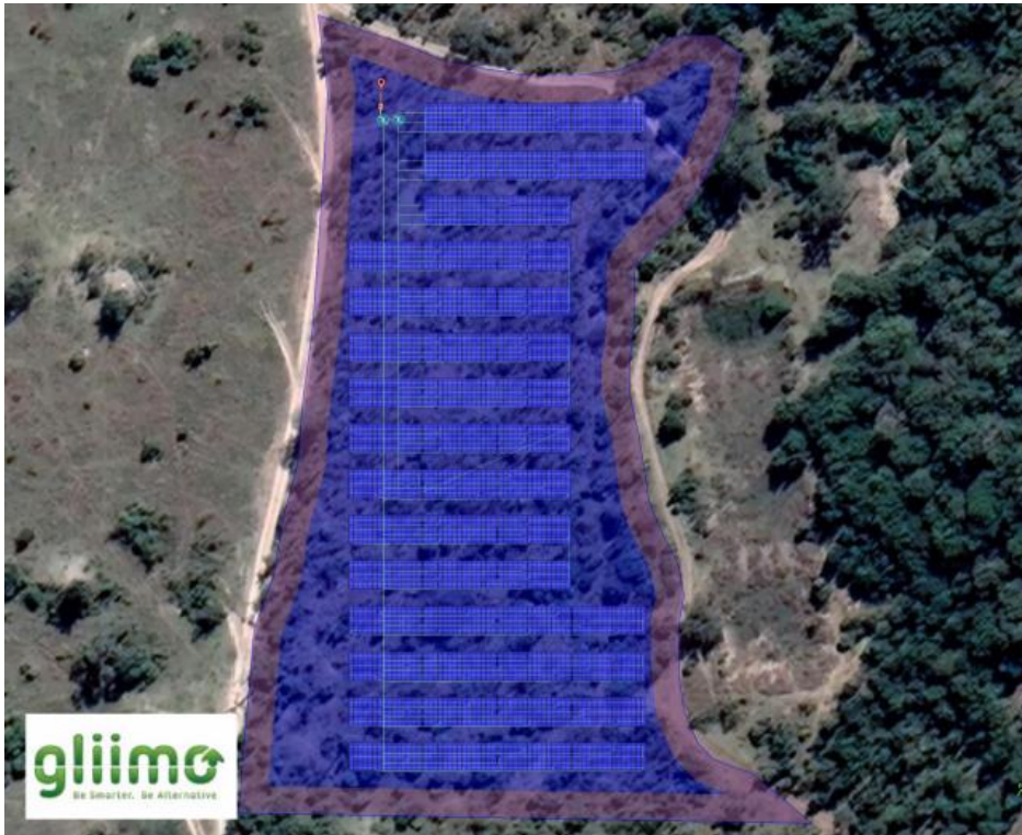
Figure 3: Layout plan for the solar banks within the full array on site Option A.
