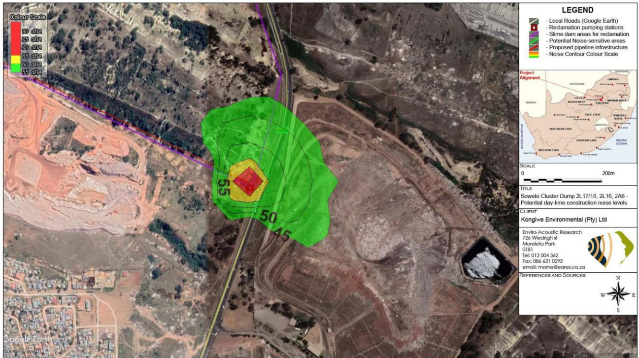
Figure 7-54: Projected conceptual daytime construction noise levels – Pump station infrastructure at Dump 2L17/18, 2L16, 2A6
