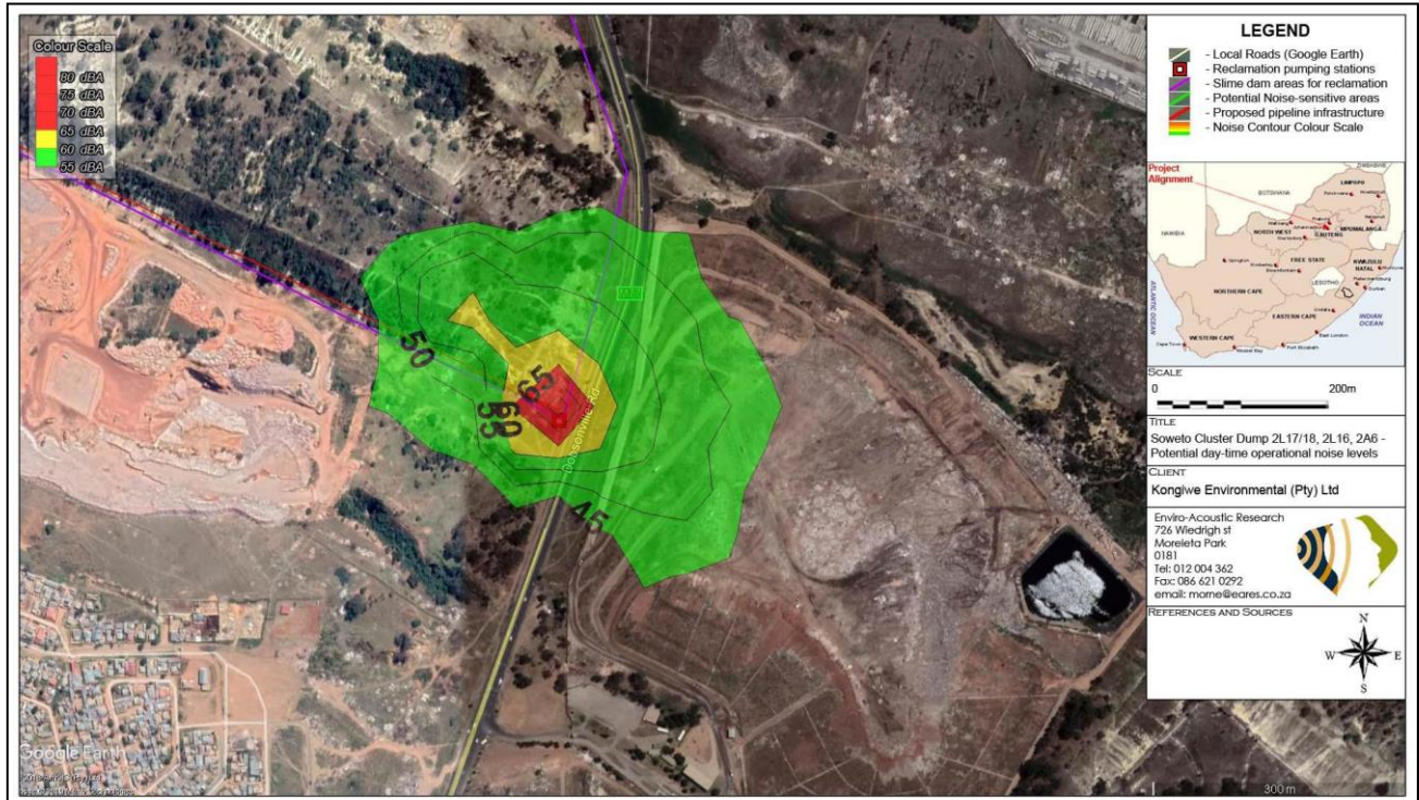
Figure 7-57: Projected conceptual daytime operational noise rating levels – Reclamation at Dump 2L17/18, 2L16 and 2A6
