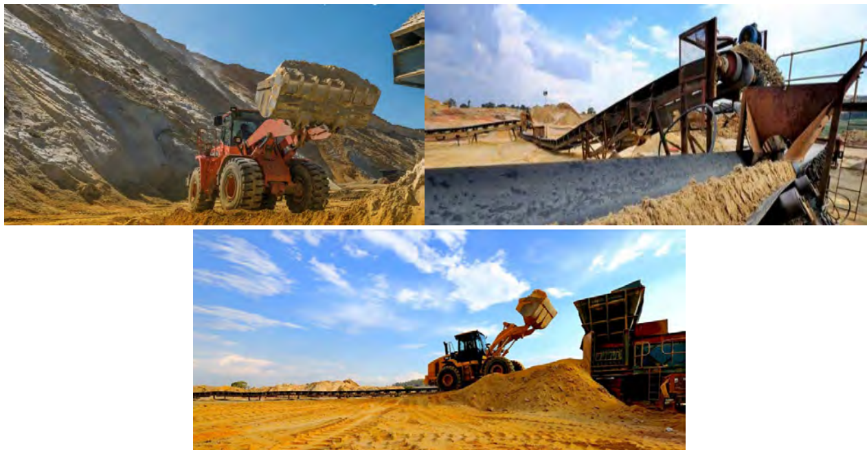
Figure 2-3: Mechanical Removal of sand from Sand Dumps. Front-end Loaders and a conveyor in operation
