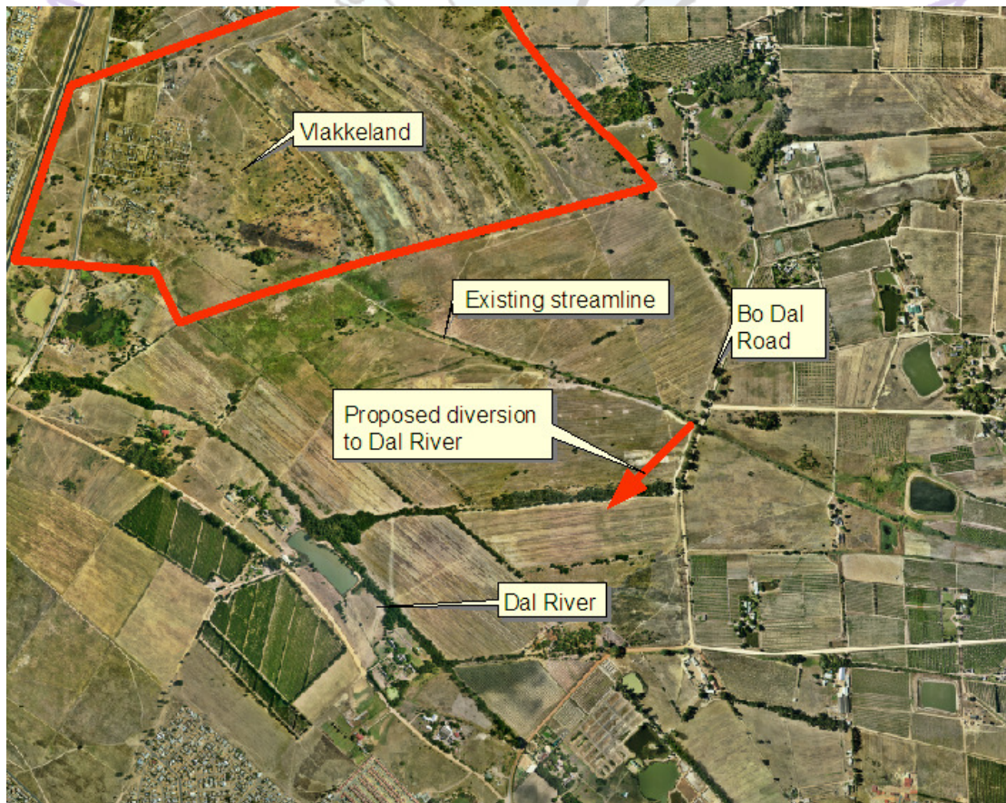
Figure 6: Proposed diversion option for the Kleinbosch Stream (Red Arrow), southwest to an adjacent, good condition drainage line flowing to the Dal River.
