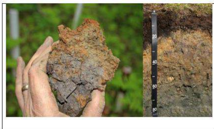
Figure 10: identification of mottles (Source: redoxymorphic feature Mottling - Bing images)
