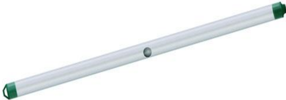
Figure 1: Bailer used to sample borehole water.
