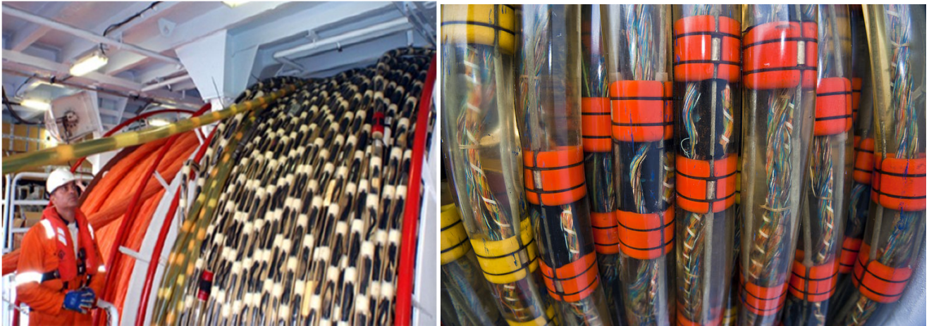
Figure 6-8: Example of a hydrophone streamer Source: (1) TEPSA and (2) https://commons.wikimedia.org/
