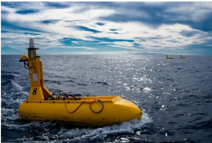
Figure 6-9: Example of a tail buoy Source: https://www.shutterstock.com/
