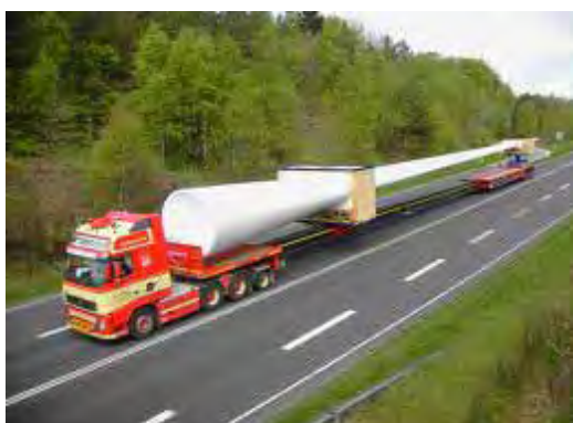
Figure 7.4: Images illustrating transportation of wind turbine components via road 11
