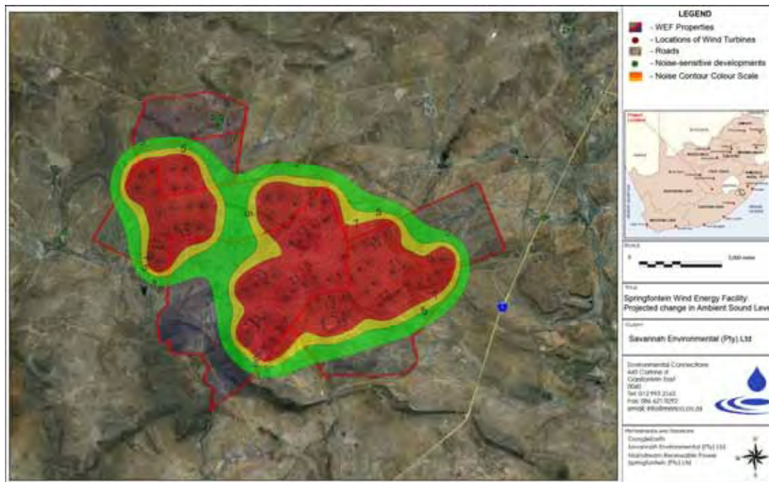
Figure 8.14: Projected change in ambient sound levels (ISO model); Contours of constant sound levels for a 6 m/s wind
