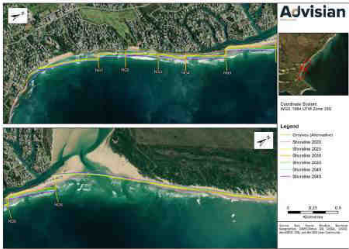
Figure 6-10: Shoreline evolution results for the Alternative general layout
