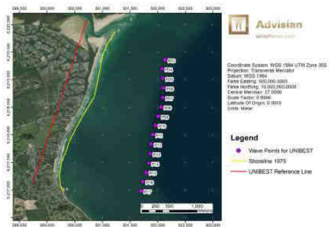
Figure 32: Location map of the local wave conditions extracted for shoreline modelling at St Francis Bay
