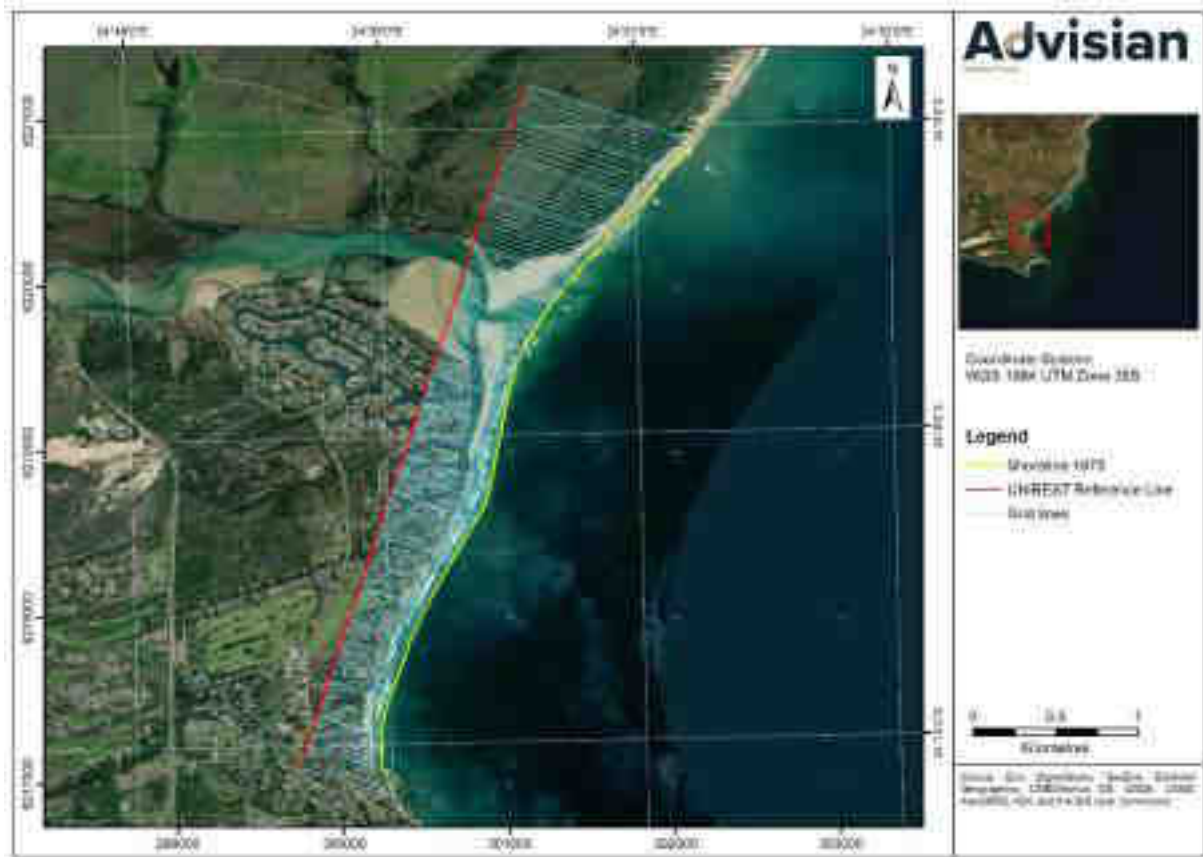
Figure 6-3: Location map of the UNIBEST-CL reference line, initial coastline and computational grid for the original shoreline model of St. Francis Bay (Advisian, 2018)
