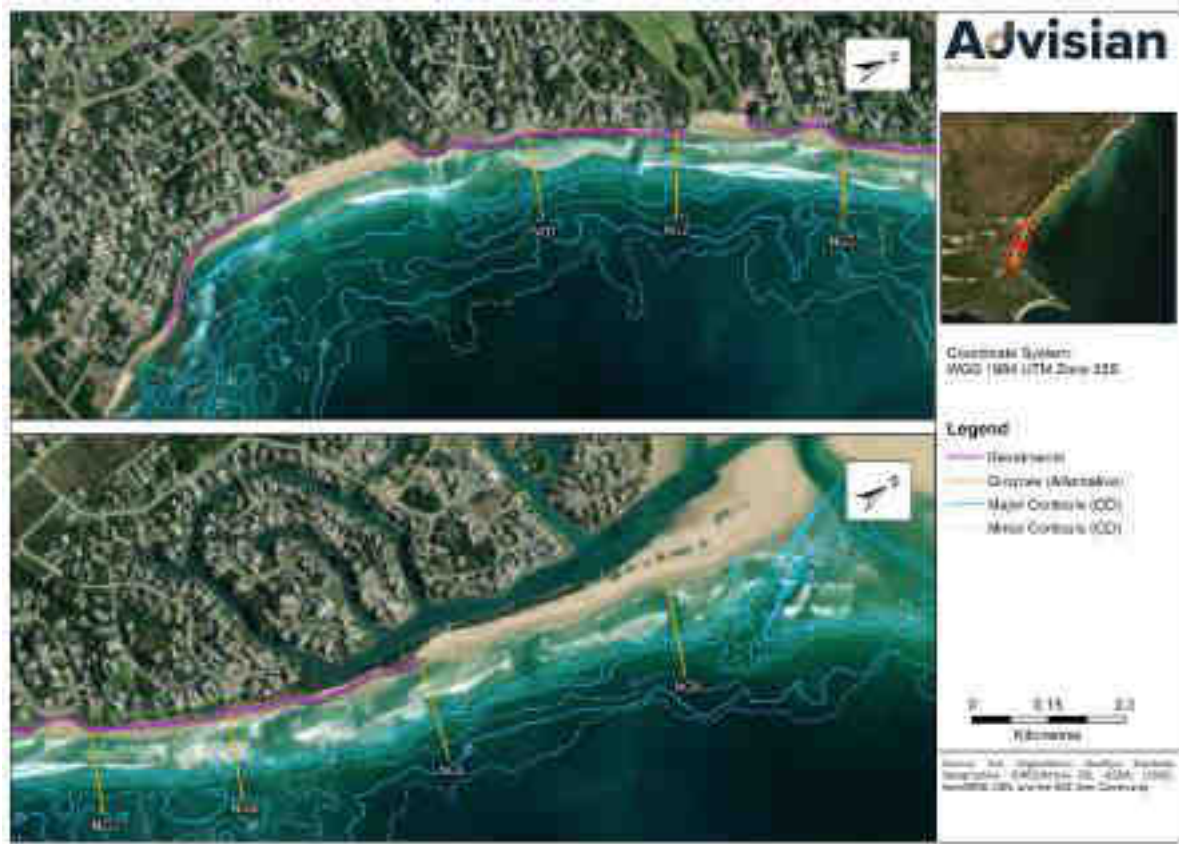
Figure 6-8: Coastal structures along St. Francis Bay shoreline for alternative protection scheme layout
