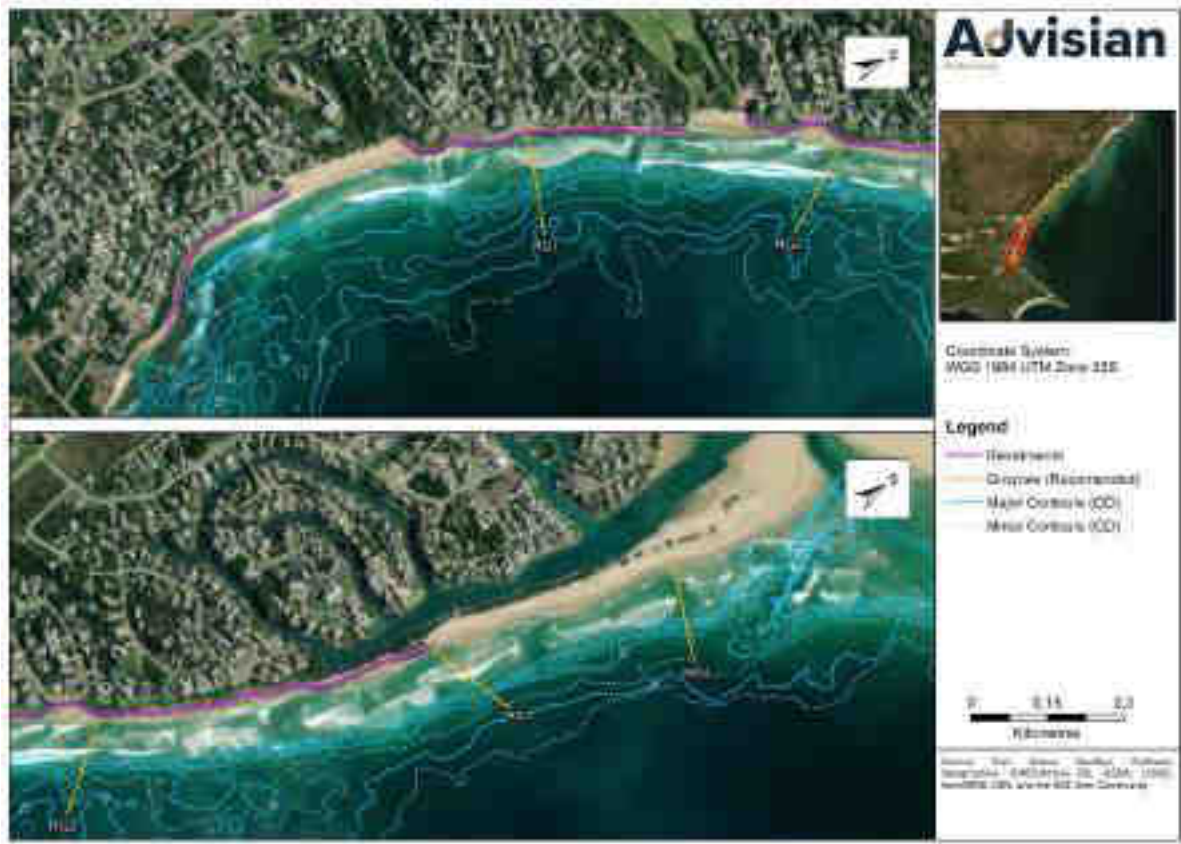
Figure 7-1: Coastal structures along St. Francis Bay shoreline for the refined protection scheme
