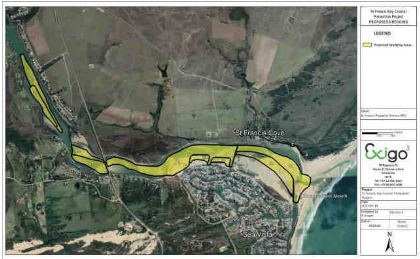
Figure 2: Aerial map detailing the extent of proposed dredging areas in the Kromme River for the proposed St Francis Bay Coastal Protection Project.
