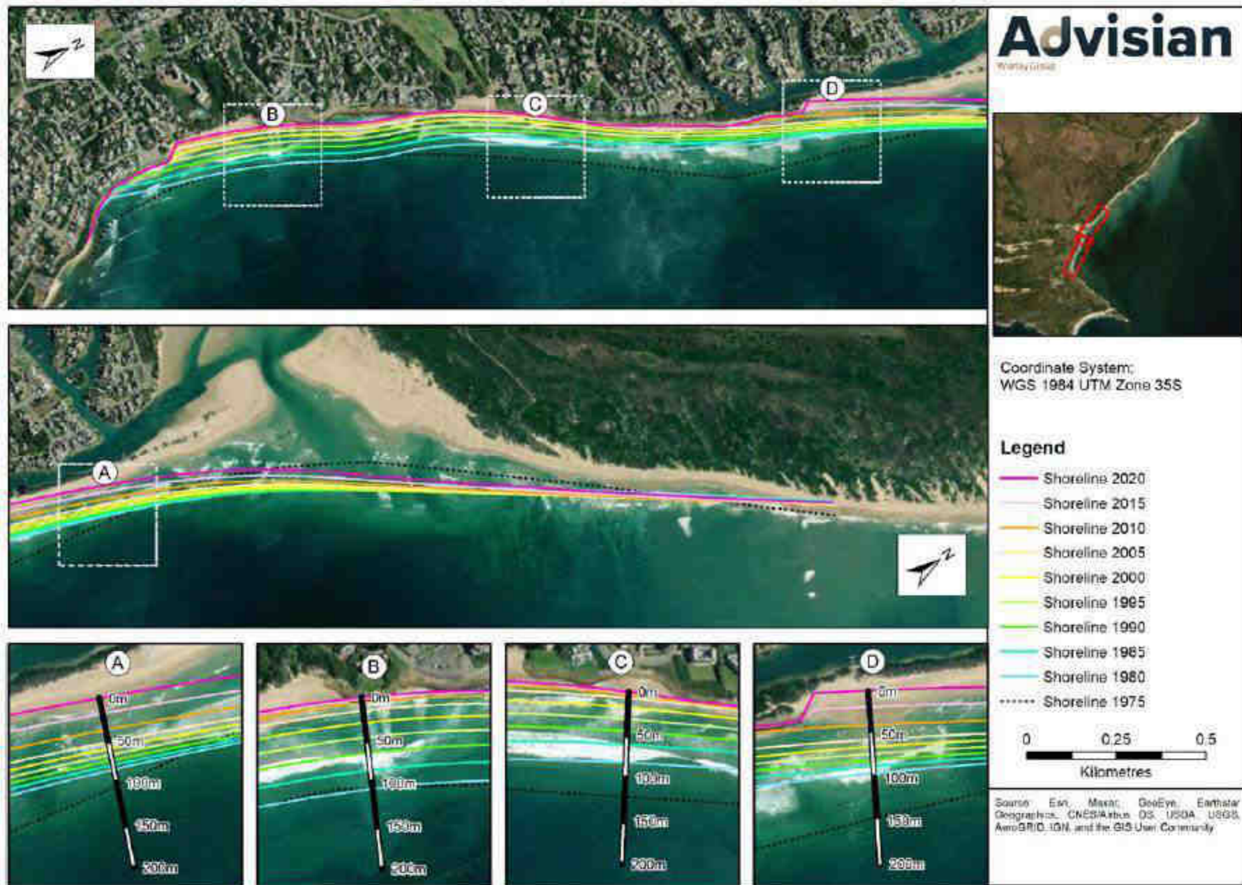
Figure 54 provides the shoreline evolution of St. Francis Bay beach for the 45-year modelling period considered (1975 – 2020)
