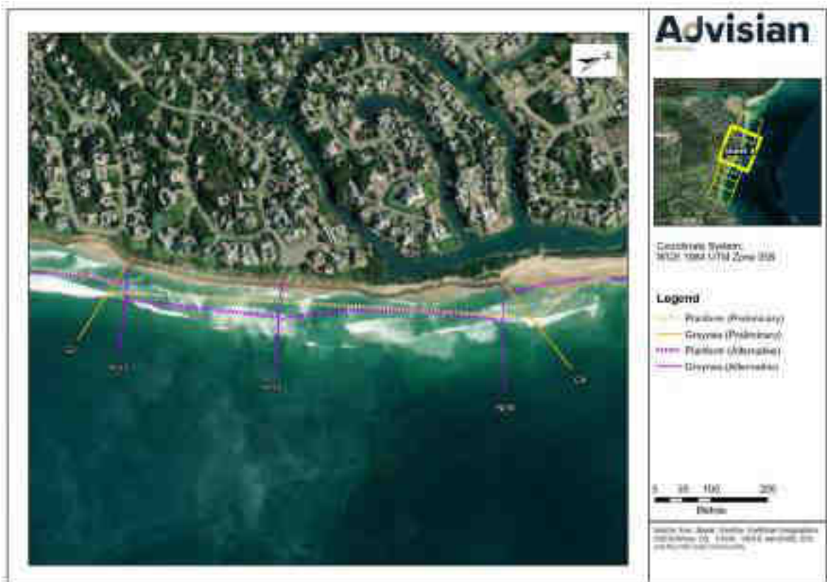
Figure 6-17: Long-term shoreline planform at the embayment between G3 (NG3) and G4 (NG5)
