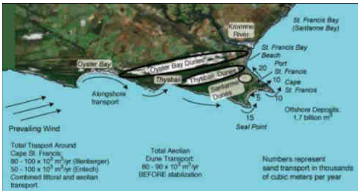
Figure 6.11: Sediment movement around St Francis Bay area (from ASR Ltd, 2006).
