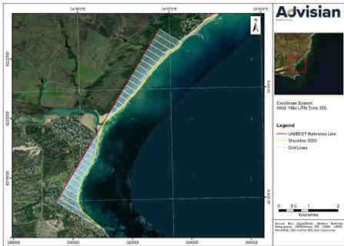
Figure 6-6: Location map of the updated UNIBEST-CL reference line, initial coastline and computational grid for the updated shoreline model of St. Francis Bay
