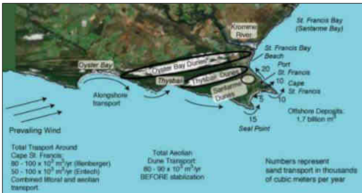
Figure 5.1: Sediment movement around St Francis Bay area (from ASR Ltd, 2006).
