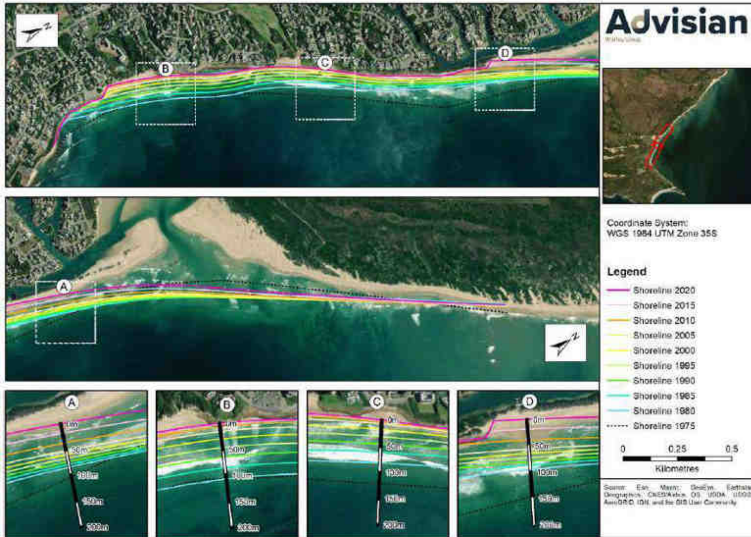
Figure 6.14 provides the shoreline evolution of St. Francis Bay beach for the 45-year modelling period considered (1975 – 2020)
