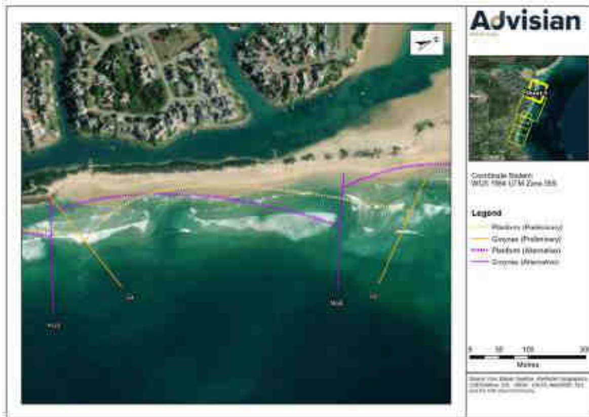
Figure 6-18: Long-term shoreline planform at the embayment between G4 (NG5) and G6 (NG7)
