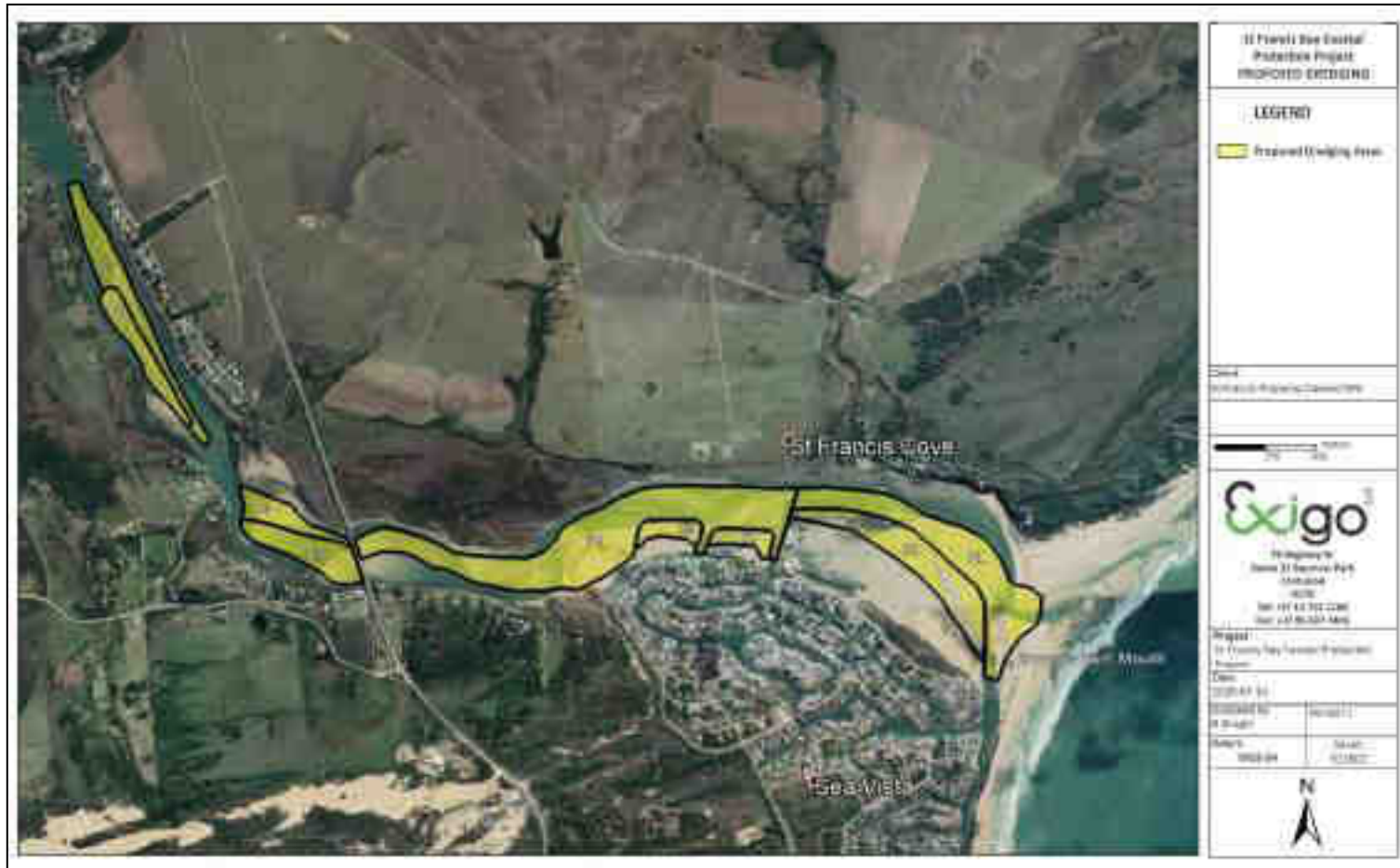
Figure 1-2: Aerial map detailing the extent of proposed dredging areas in the Kromme River for the proposed St Francis Bay Coastal Protection Project.
