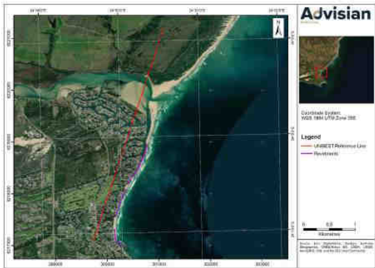
Figure 6-4: Location map of the UNIBEST-CL rock revetments for the original shoreline model of St. Francis Bay (Advisian, 2018)
