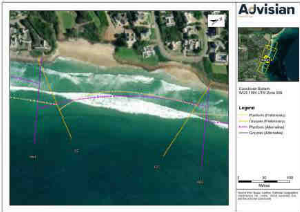
Figure 6-16: Long-term shoreline planform at the embayment between G2 (NG2) and G3 (NG3)
