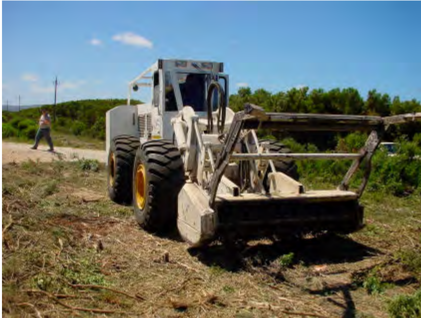
Figure 2. An example of a mechanical mulching machine.
