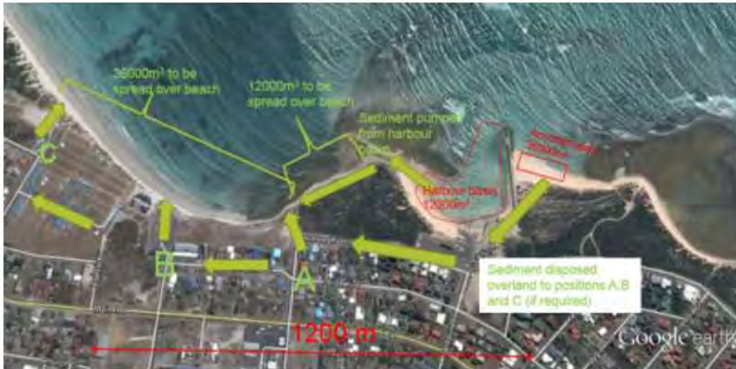
Figure 15: Proposed dredging plan for the Struisbaai harbour and accreted sediment removal at the east beach and the proposed disposal/beach nourishment location on west beach
