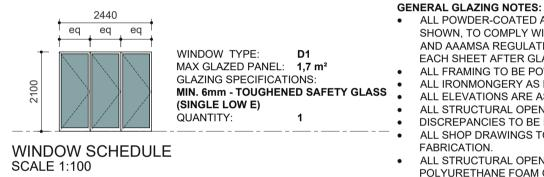
• ALL POWDER-COATED ALUMINIUM DOORS & WINDOWS WITH GLAZING PANELS AS SHOWN, TO COMPLY WITH SANS 1263:1, SANS 0137, SANS 10400 PART N SCHEDULE 1 AND AAAMSA REGULATIONS; WITH MANUFACTURE-NAME PERMANENTLY MARKED ON EACH SHEET AFTER GLAZING.
