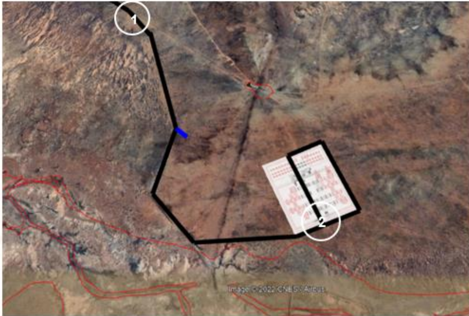
Figure 1. Section of new road from its intersection with the existing private road/farm track (1) to the Main Transmission Substation MTS (2). A short access road to the Switching Station (Dx) will also be developed (blue line). Red lines indicate flood plain soils (possible watercourse).
