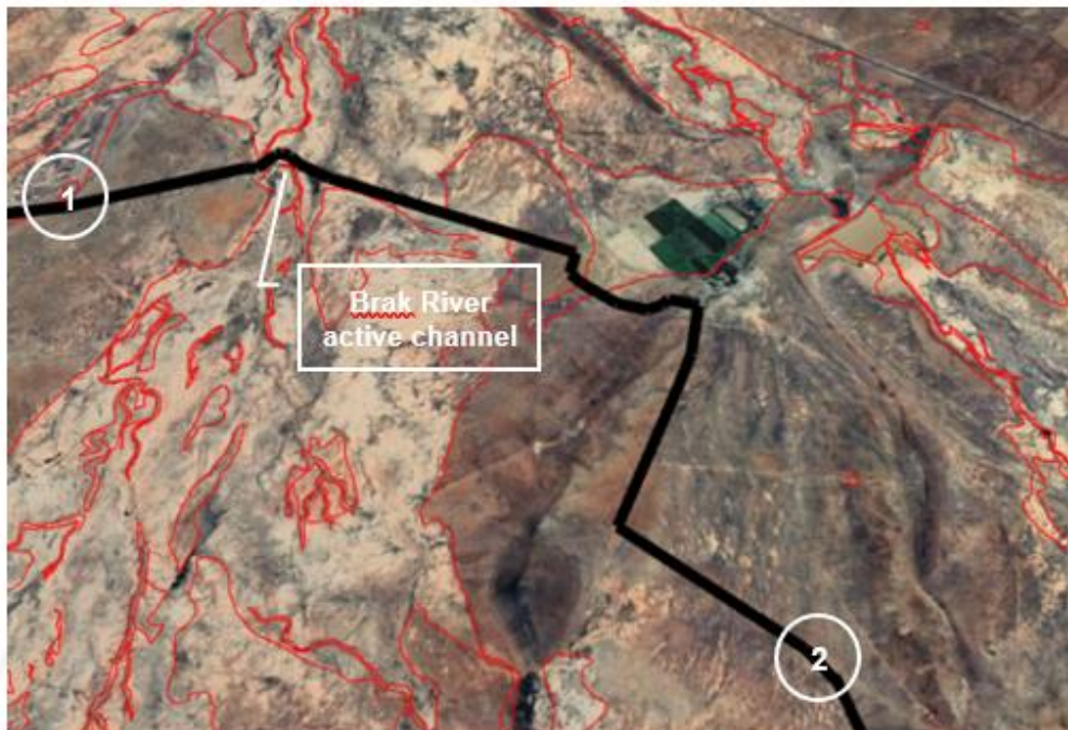
Figure 1. Section of existing private road from its intersection with the 'Burgerville' District Road (2448) at the farm boundary (1) to its intersection with the new road (2). Red lines indicate flood plain soils, including the Brak River.
