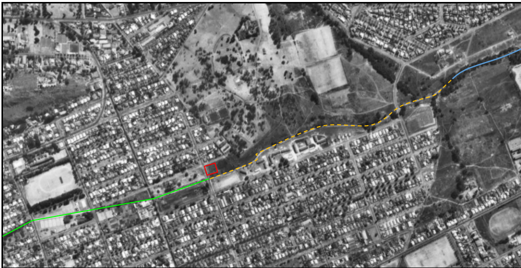
Figure 3: Historical imagery (circa 1962), indicating the extensive residential development surrounding the Bezuidenhout Valley Clinic property (red square), the canalised portion of the Jukskei River (orange line) joining to the natural watercourse (blue line). The green line indicates an underground portion of the canal which daylights at the south-western corner of the clinic property.
