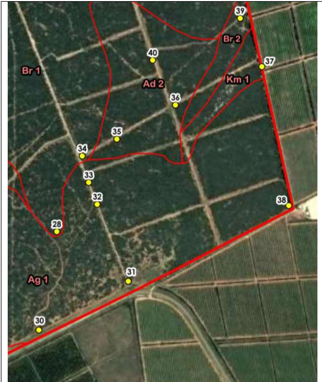
Map 5.1 Location of the soil pits on the cleared 20.2 ha. The yellow dot and corresponding number indicates the soil pit and the map symbol, e.g. Ag1 indicates the soil type
