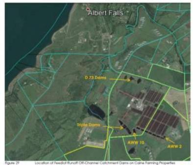
Effluent from the abattoir is directed to a series of ten offchannel maturation ponds, the first five ponds are anaerobic and the second five are aerobic. Treated water from the tenth dam is pumped to Back Dam (near the R614) and Wondervale (adjacent to the D73 near the former poultry farm), or directly to lands for irrigation.
