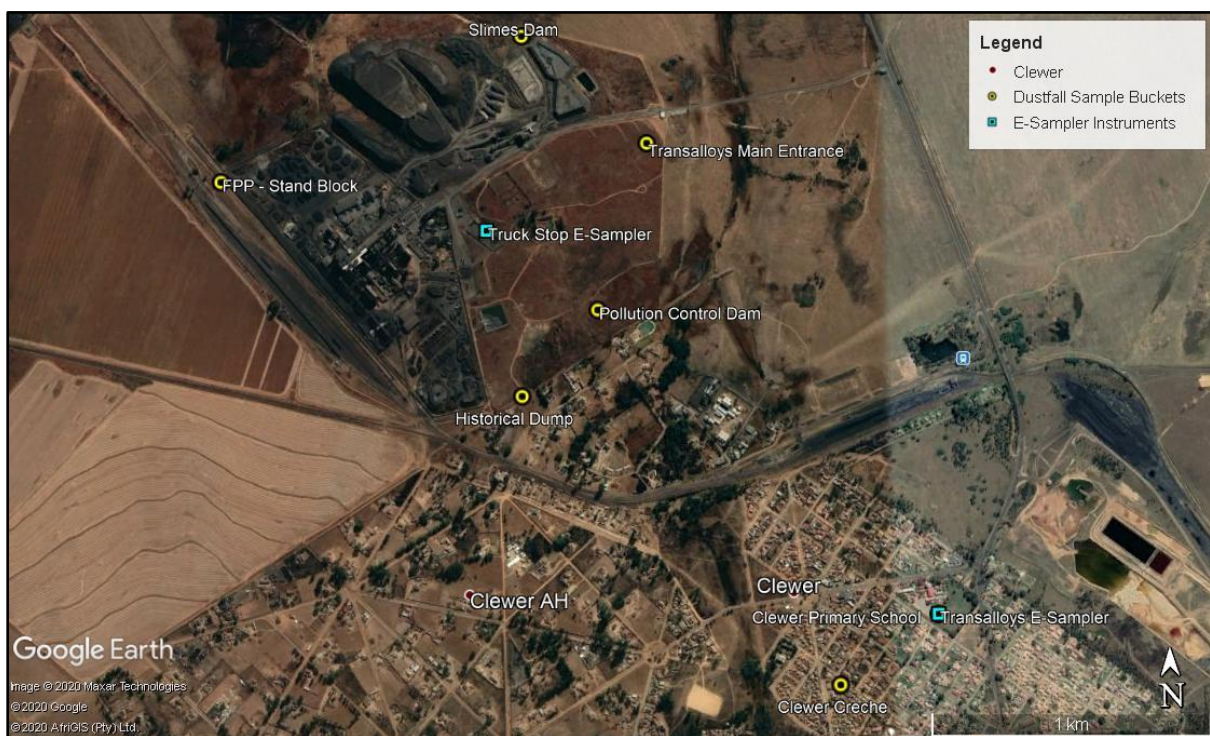
Figure 10-4: Transalloys' dust and PM 10 monitoring points (Skyside, 2021)
