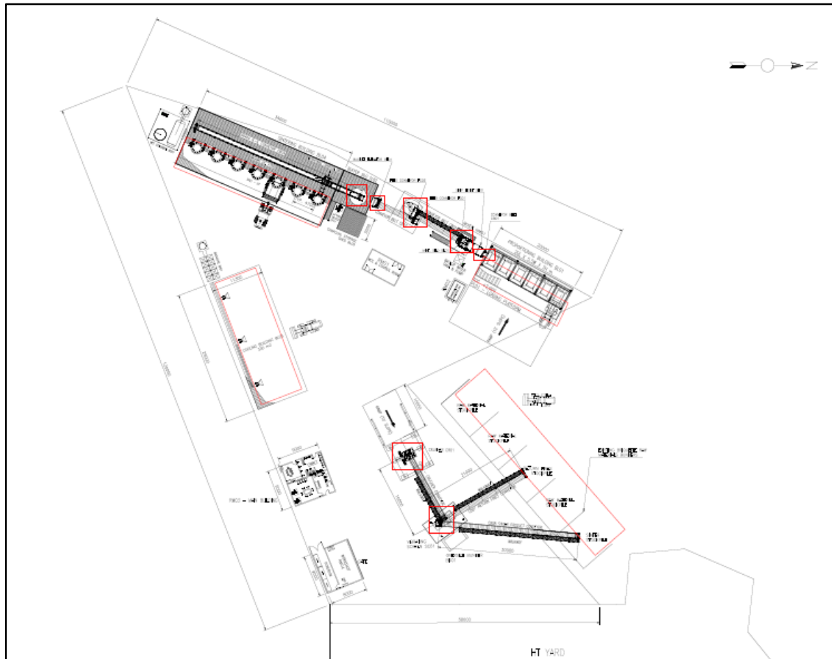
Figure 7-4: Layout 4 (preferred based on preferred position – area of briquetting raw material bunkers)
