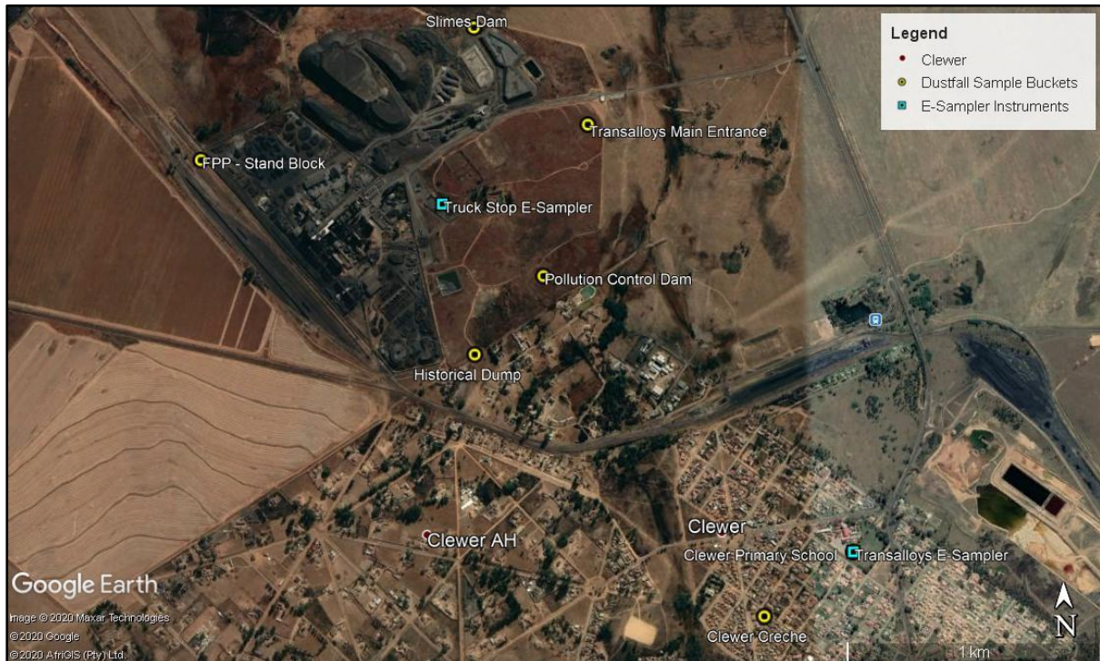
Figure 10-4: Transalloys’ dust and PM 10 monitoring points (Skyside, 2021)
