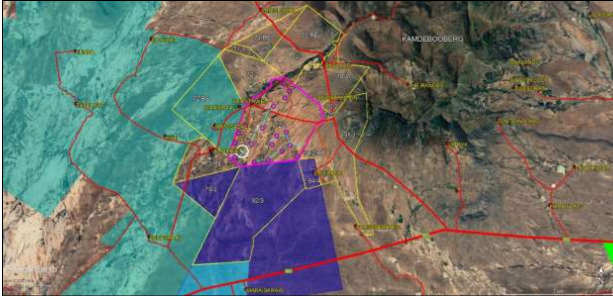
Figure 3.5: FE Tango WEF site (pink outline) in relation to adjacent properties (yellow) and existing roads (red). Also indicated are proposed FE Tango turbines (pink circles), substation hub (white fill, circled white), proposed roads (light blue lines). Dark blue fill indicates Eskom’s approved Aberdeen WEF (dark blue fill), and concurrently proposed Kariega 1-4 WEF cluster (light blue fill) (Source: Chief Surveyor-General) 13 .
