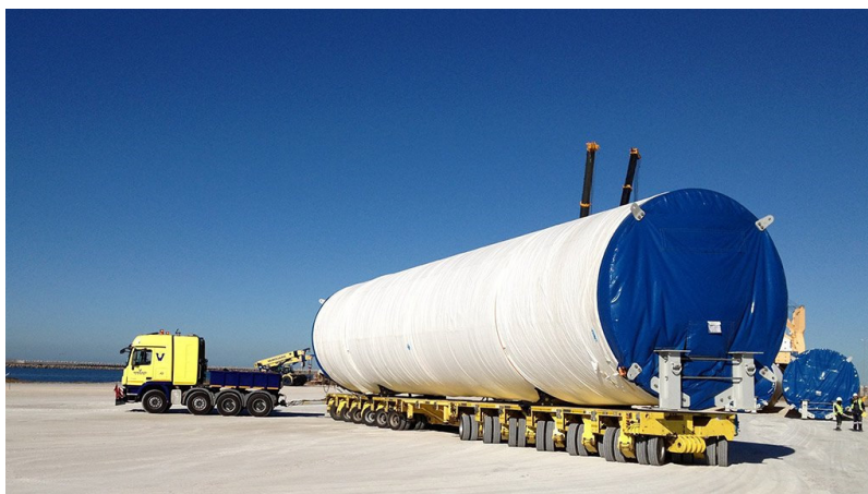
Figure 4-3: Transporting the Tower Sections (Montiea, 2014)
