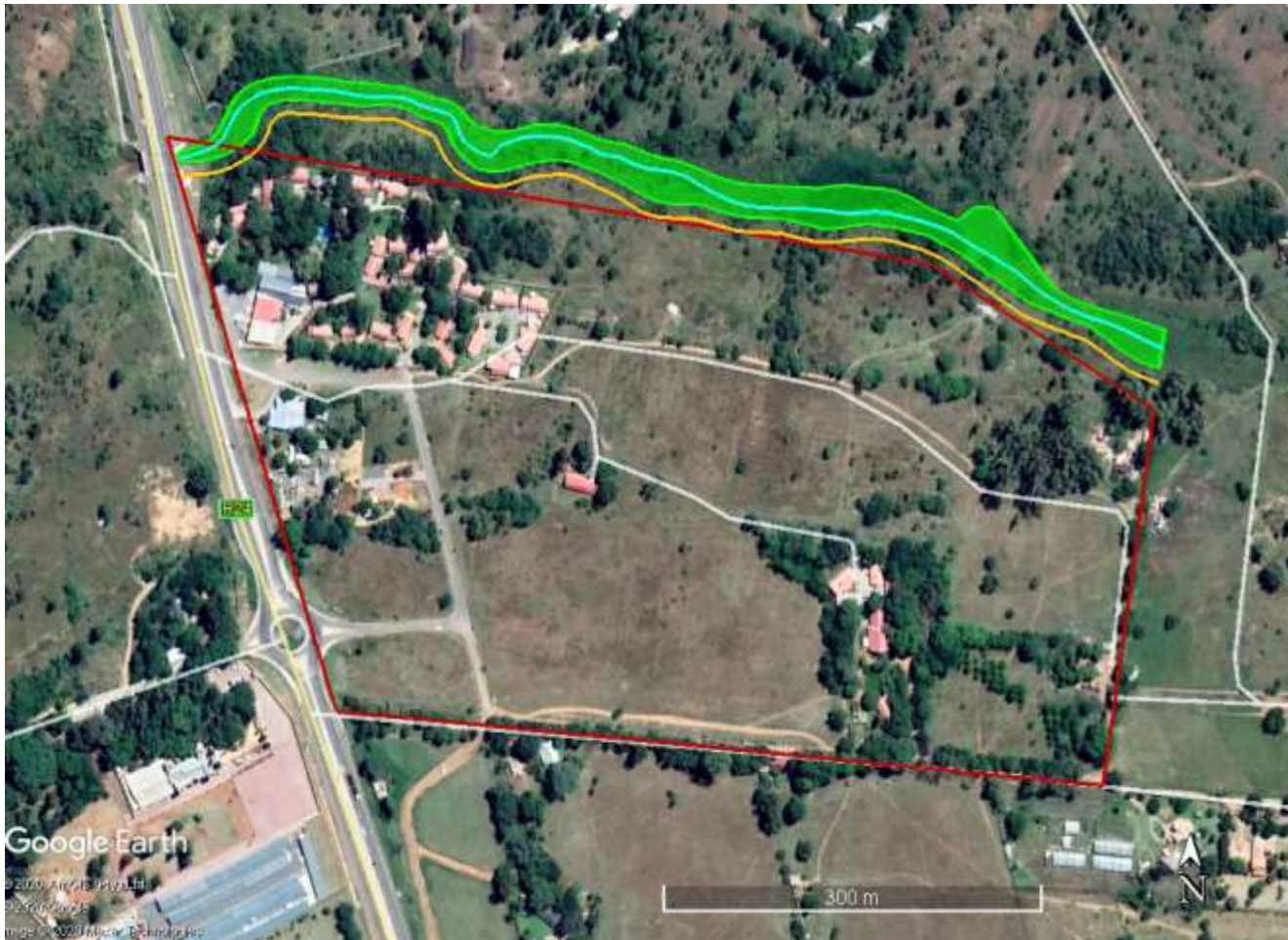
Figure 2 Indication of non-perennial river (active channel, riparian zone, buffer zone) that enters the northwestern corner of the site as well as running outside the northern boundary of the site.
