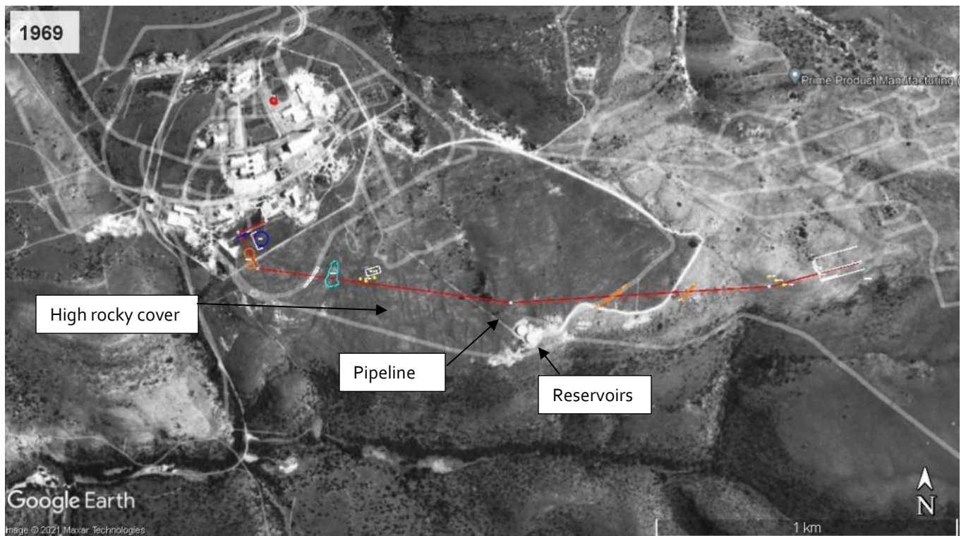
Figure 8: Historic aerial image dated 1969 of the area that the route is situated in. To geofence the image, it was superimposed on Google Earth
