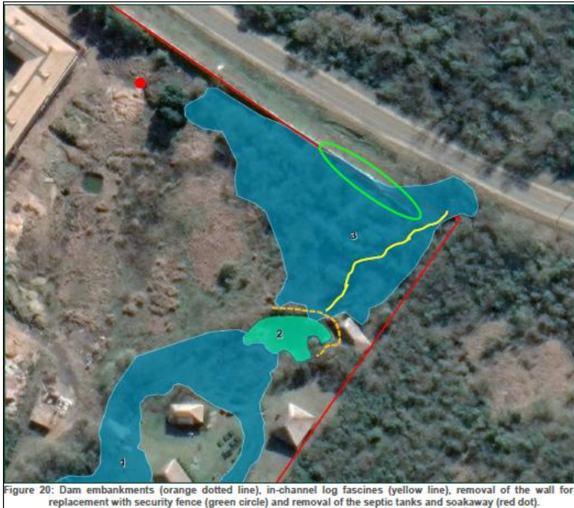
Figure 8: HGM Units 2 & 3 Rehabilitation Recommendations (Kinvig & Associates).
