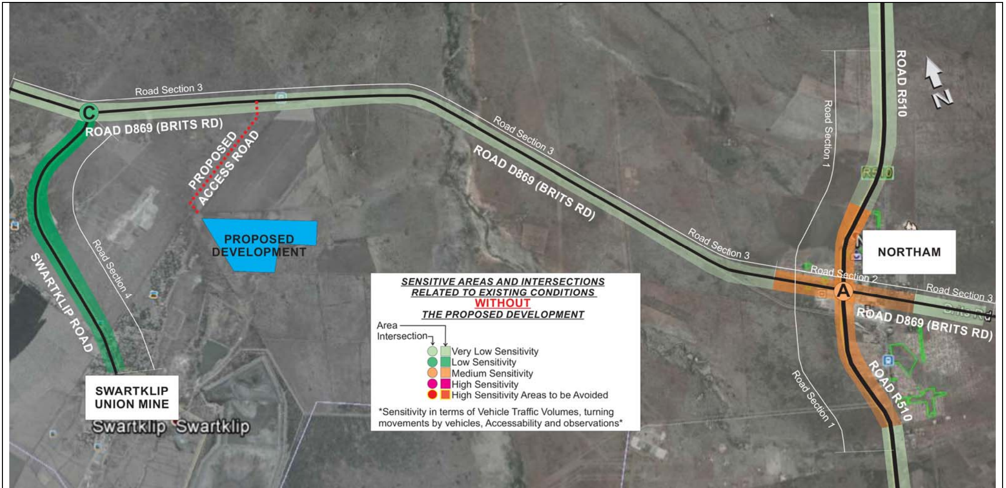
FIGURE 2.3: SENSITIVE ROAD SECTIONS AND INTERSECTIONS RELATED TO EXISTING CONDITIONS WITHOUT THE PROPOSED DEVELOPMENT
