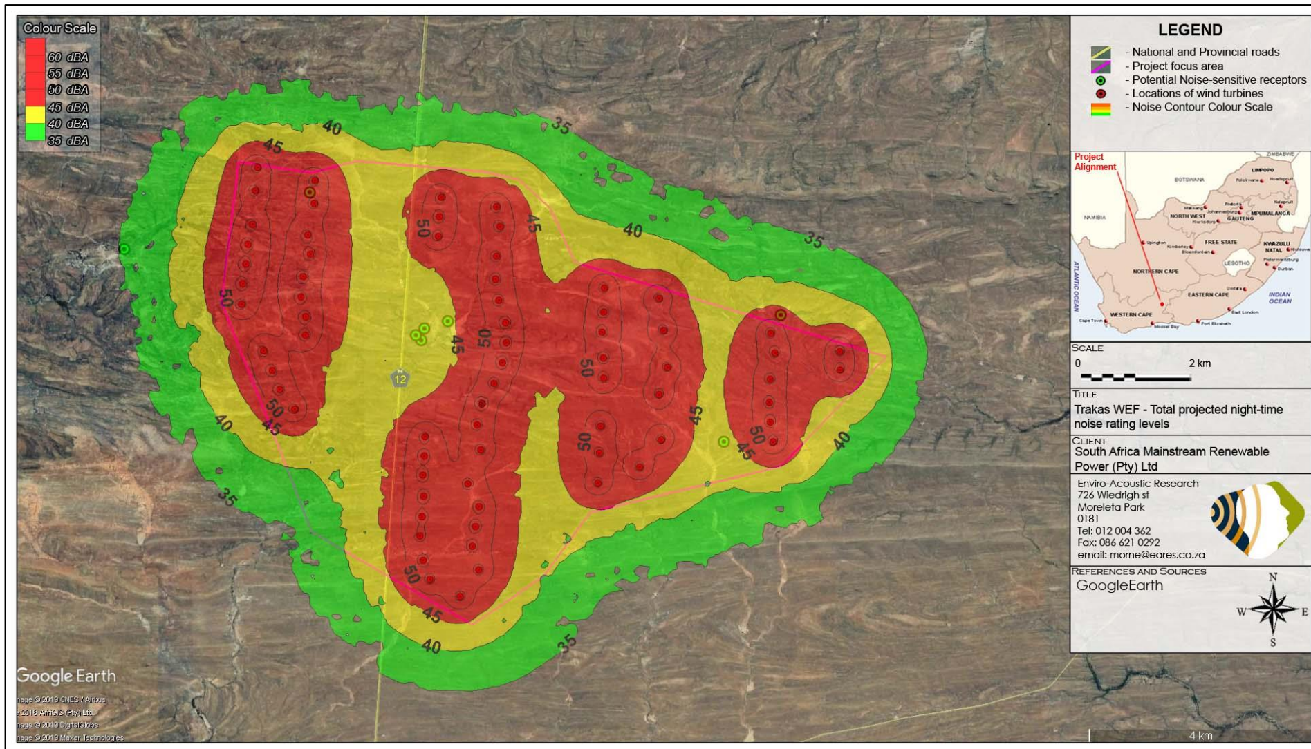
Figure 10-2: Projected conceptual night-time noise rating levels of the Trakas WEF during operation
