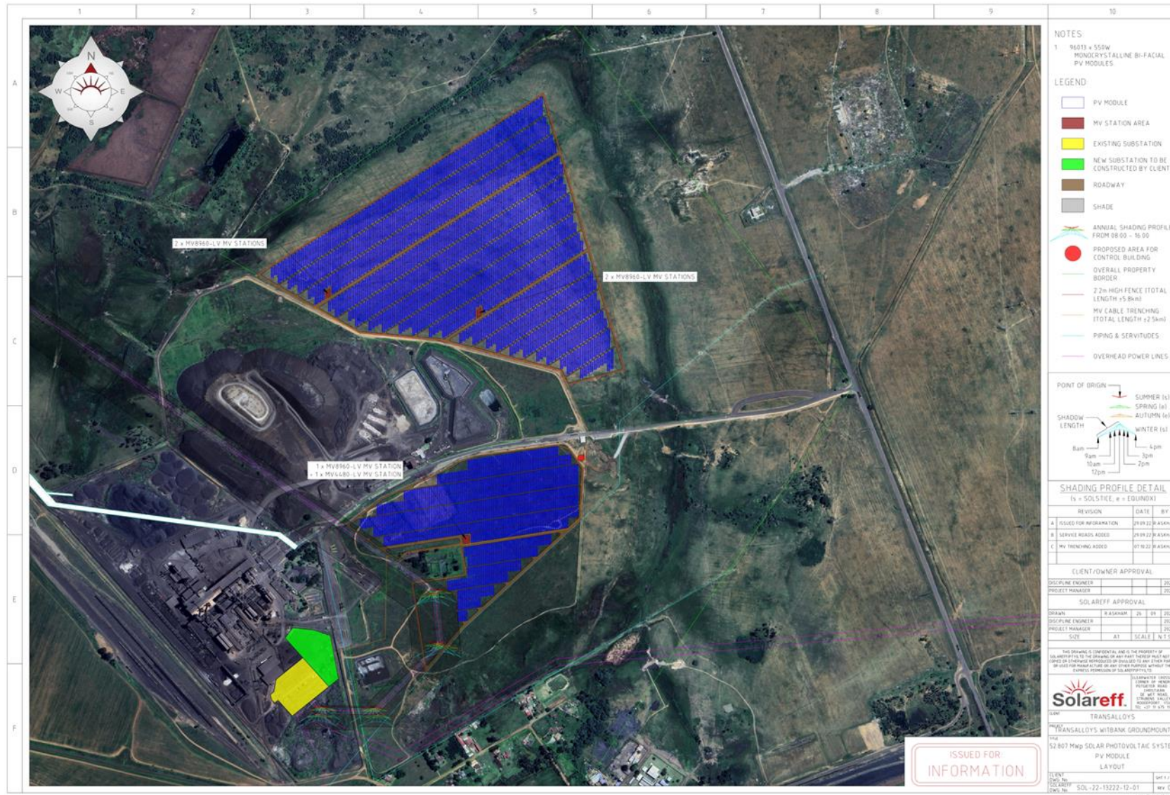
Figure 1.2: The entire extent of the development footprint (~67.9ha) layout as assessed within this BA Report for the Transalloys Solar PV Energy Facility
