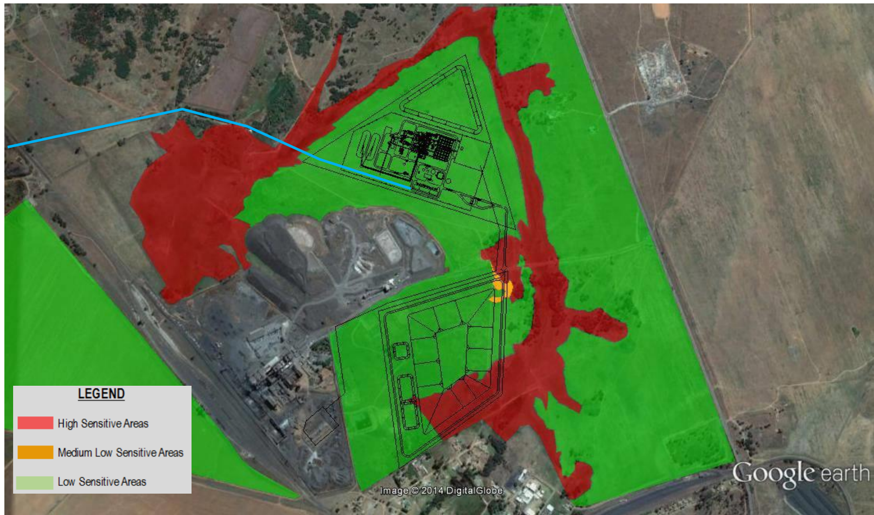
Figure 7.2: Ecological sensitivity map indicating overlay of 150MW power plant. 50MW plant would be restricted to northern site (triangle)
