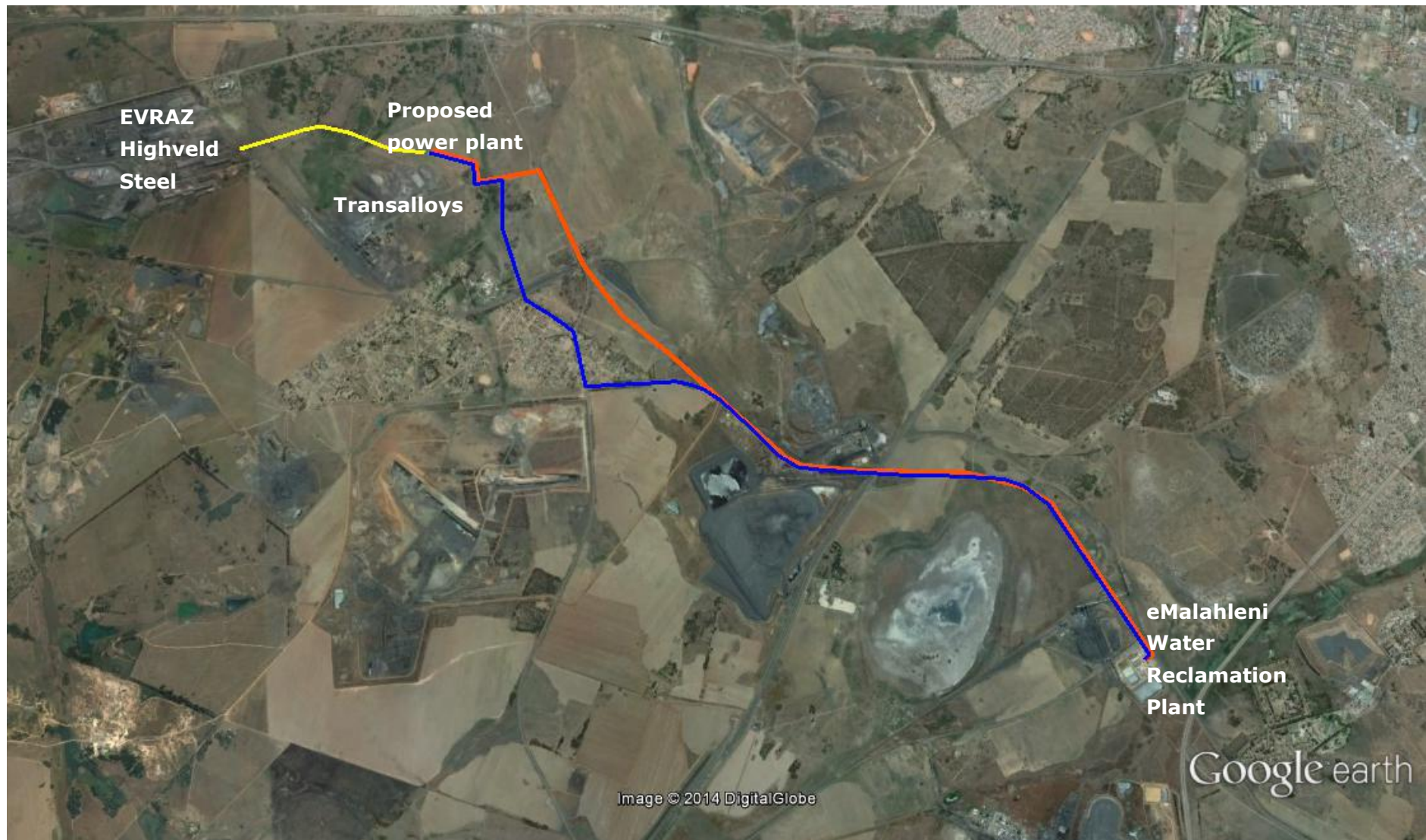
Figure 4.3: Water pipeline route alternatives. The orange line and blue lines represent route options 1 and 2 from the project site to the EWRP over Landau Colliery surface rights area. The yellow line represents the route between project site and Highveld Steel
