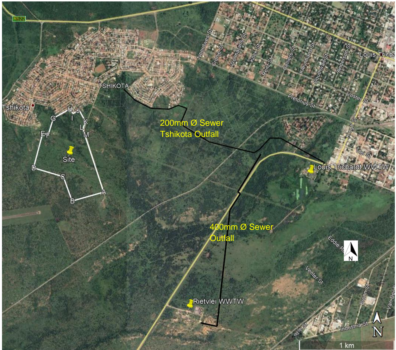
Figure 10 Existing sewer outfalls
