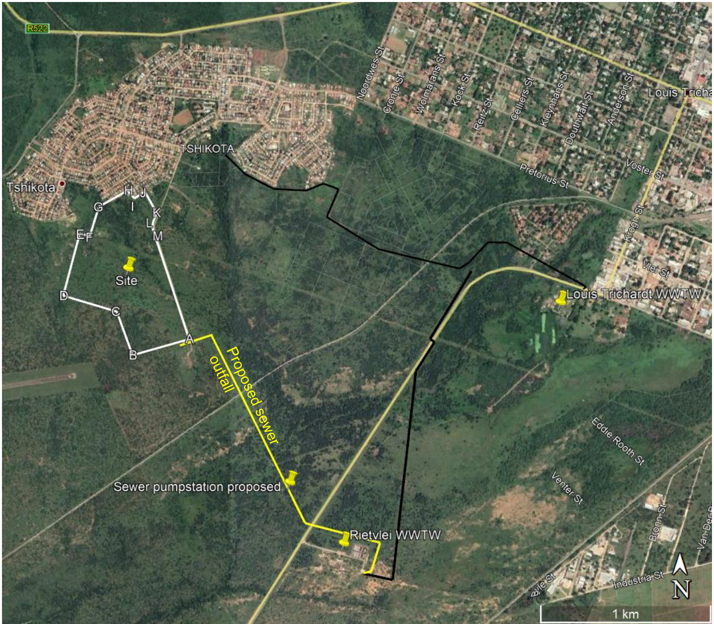
Figure 11 Proposed sewer outfall
