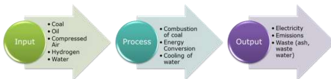
Figure 3.2: Resources (input), processes and outputs (waste) for a coal-fired power station
