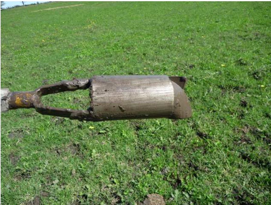
Figure 6 Striking of soil on soil auger – no soil could be extracted from the sample pit
