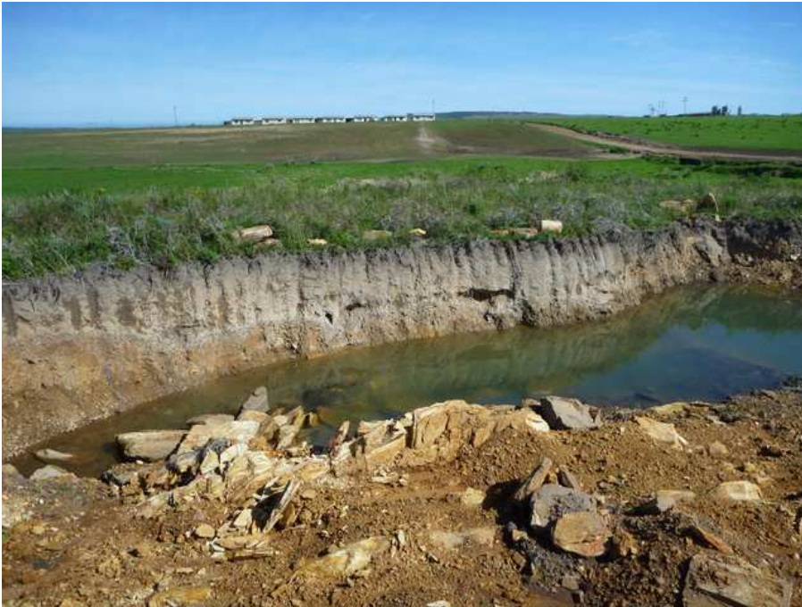
Figure 18 Exposed profile of variable depth sandy soils of different soil forms (Glenrosa, Cartref and Houwhoek).
