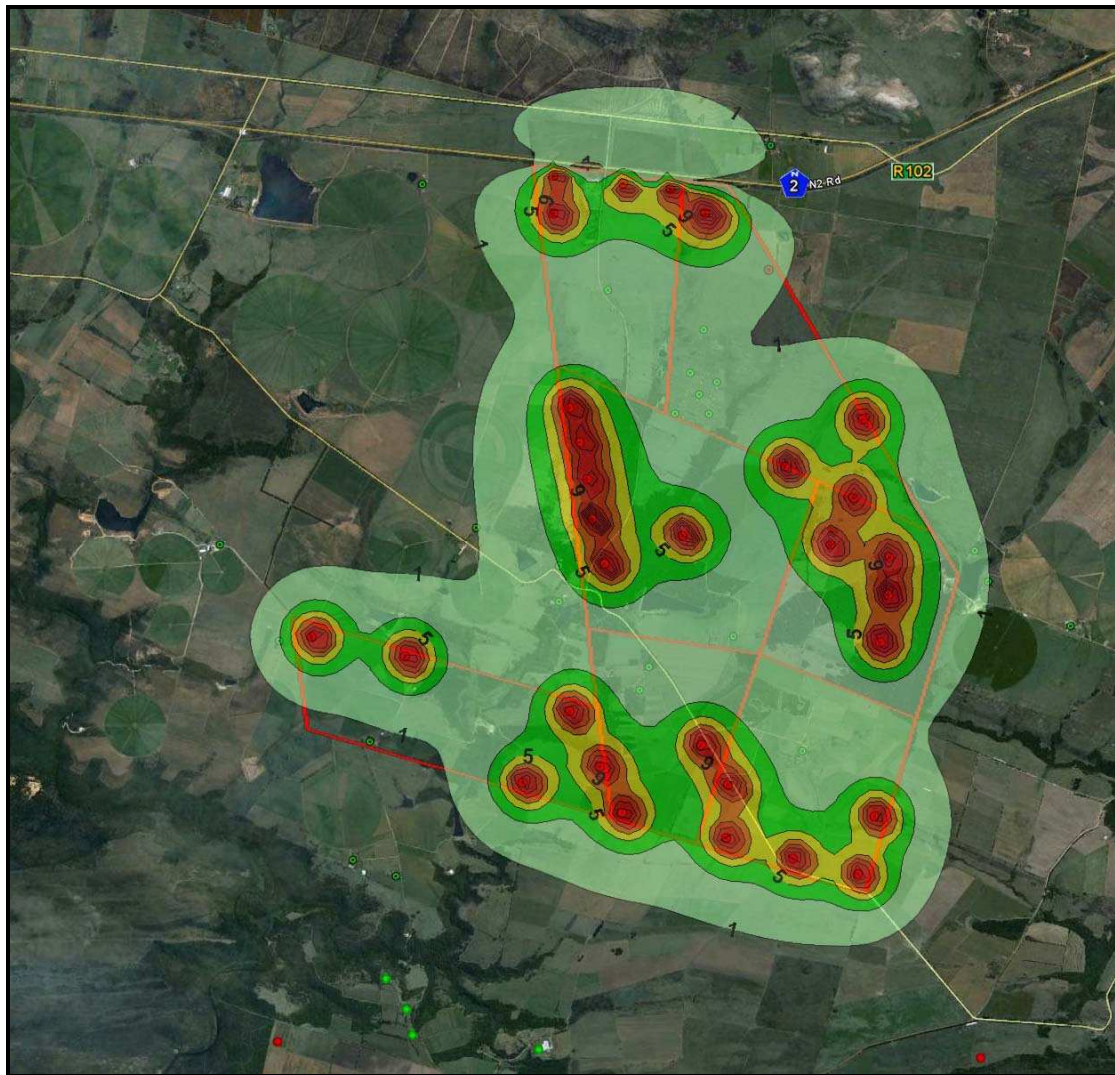
Figure 7-6: Change in ambient sound levels (ISO model), contours of constant noise levels for a 5 m/s wind (turbines marked as red dots, NSDs as green dots)
