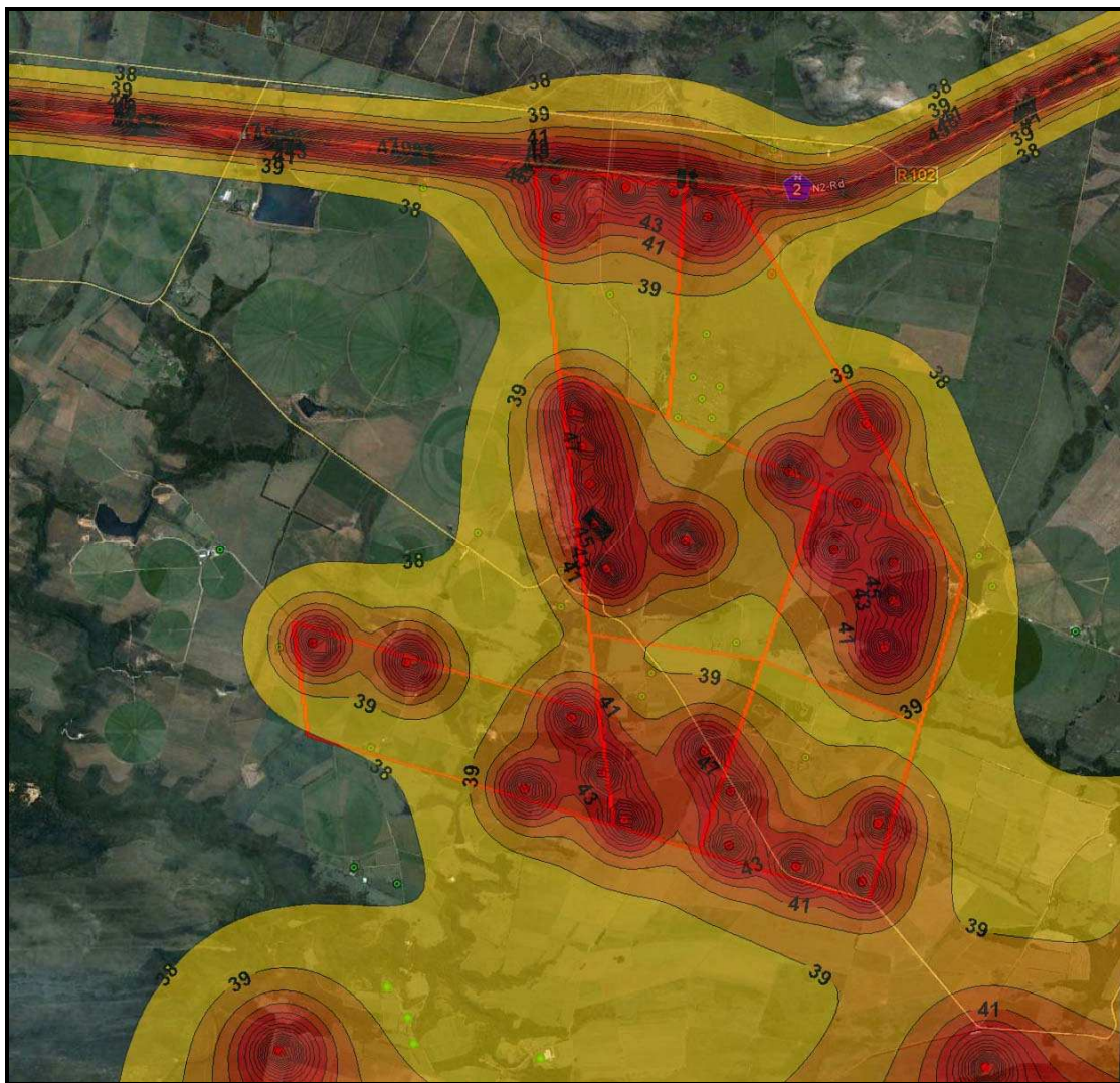
Figure 7-5: Total Projected Sound Levels (ISO model) from facility; Contours of constant sound levels for a 5 m/s wind (WTGs marked as red dots, PSRs as green dots)
