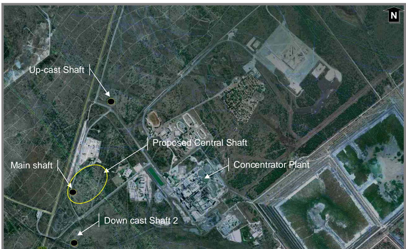
Figure 5: Layout Map of existing and proposed shaft sites
