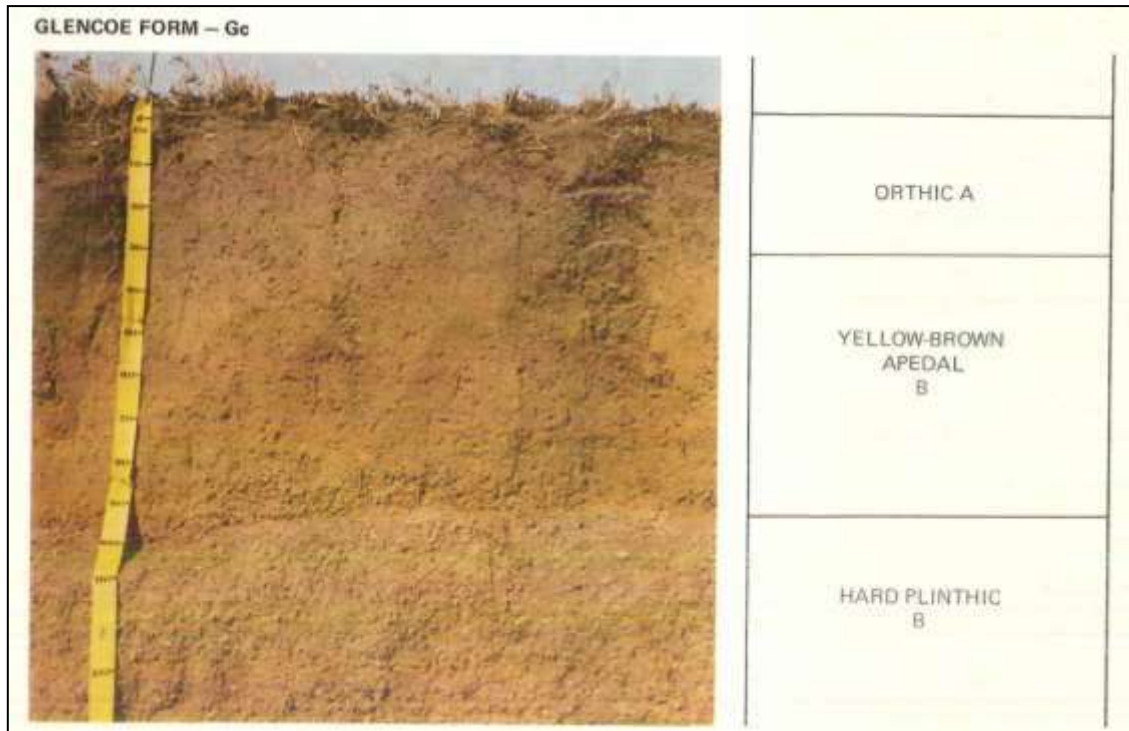
Figure 10-19: A typical cross section for the Glencoe soil form (Soil Classification Working Group, 1977)
