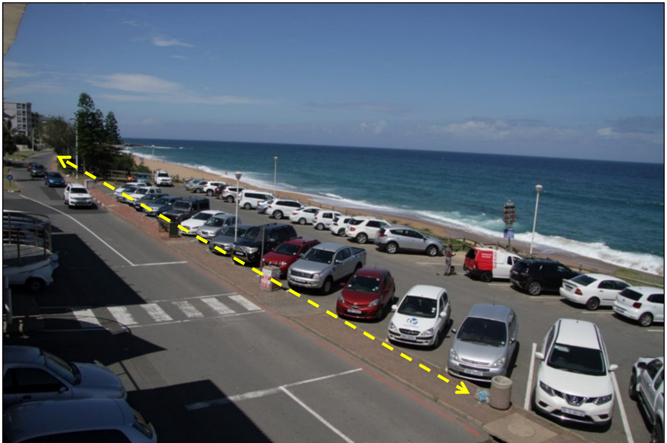
PLATE 7-1: The approximate alignment of the proposed in-situ culvert to be constructed below the pedestrian walkway adjacent to the parking lot.
