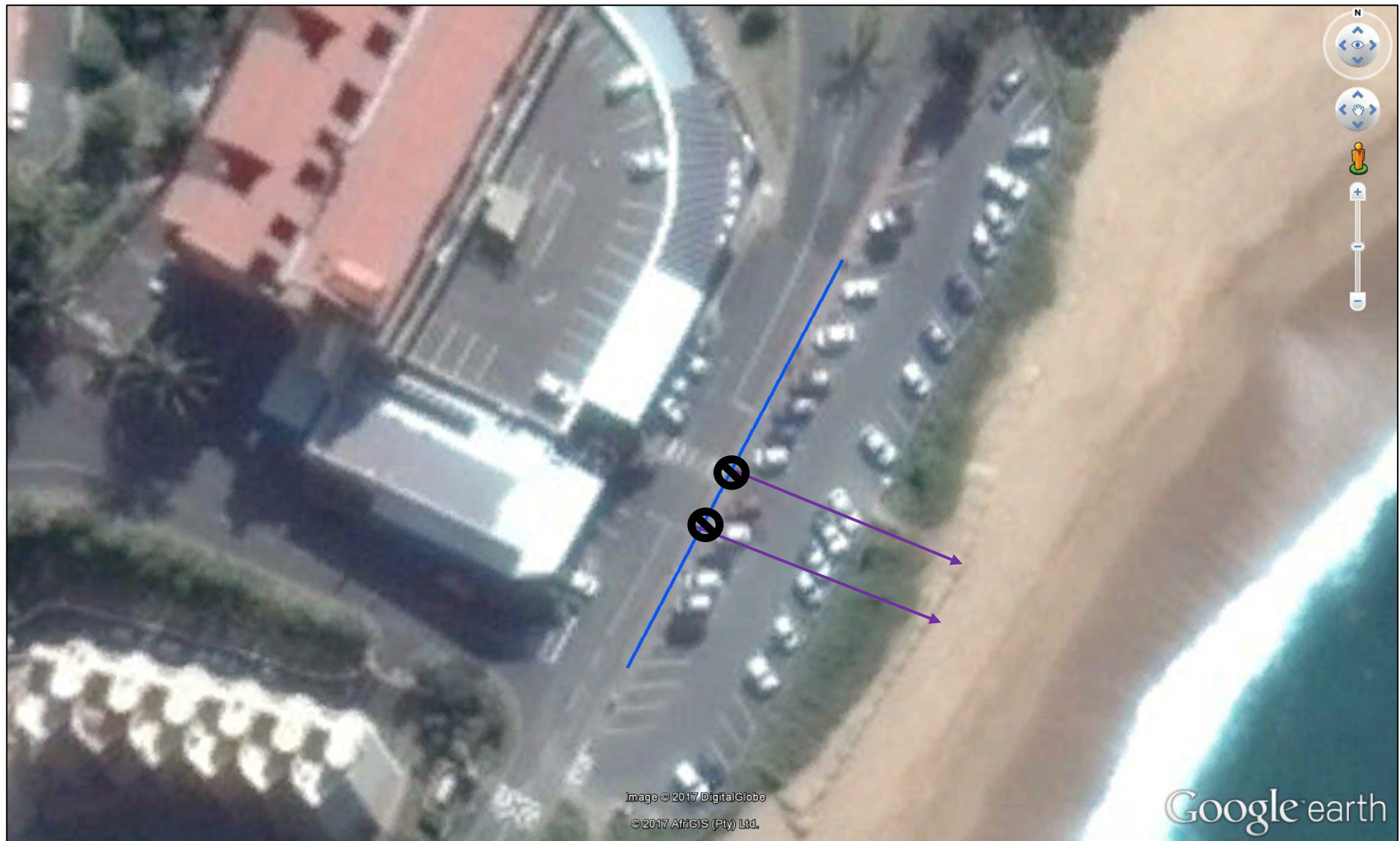
FIGURE 4-3: The points at which the existing stormwater outlets (illustrated in purple), which intersect with a portion of the existing stormwater pipeline (illustrated in blue) will be blocked off and abandoned.
