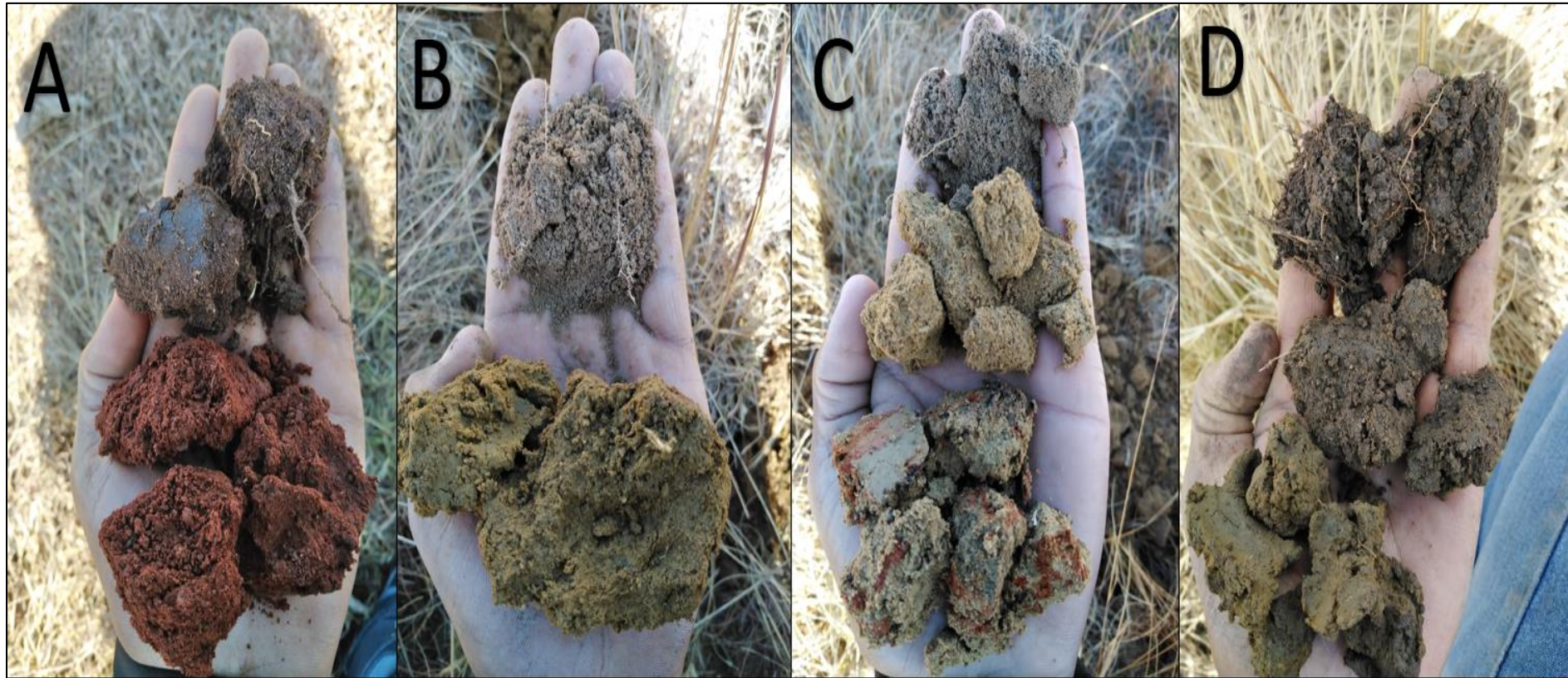
Figure 6-1 Dominant soils identified during the site assessment. A) Red apedal horizon. B) Yellow-brown apedal horizon C) Orthic on top of yellow-brown apedal, underlined by soft-plinthite (Avalon). D) Orthic on top of neocutanic, over gley horizon.
