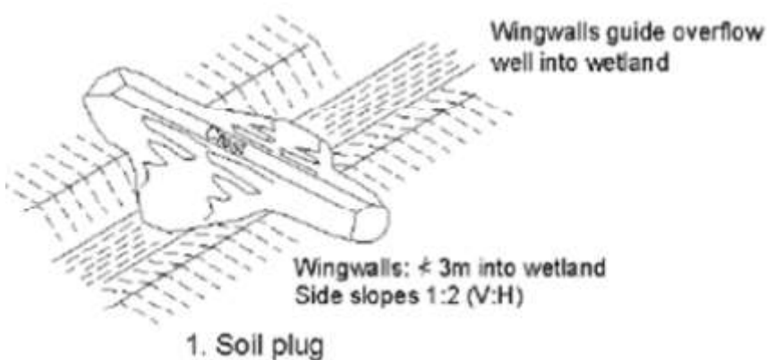
Figure 3-3 Example of an 'earth plug' (Russell, 2009)
