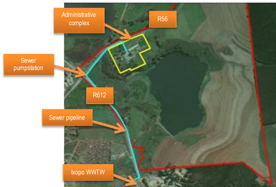
Figure 8: Proposed alternative routing of sewer pipeline between administrative complex and Ixopo WWTW
