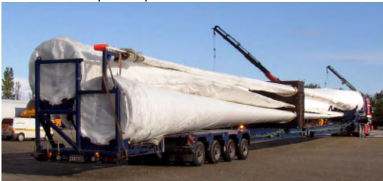
Plate 2: 3 x 45 m Blades on extendible Trailers
