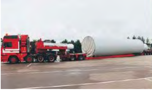
Plate 3: 20 m Tower Section on low-bed tri-axial Trailer (Very little ground clearance)
