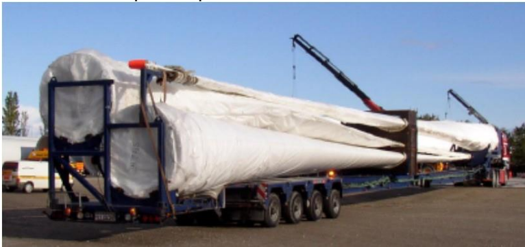
Plate 2: 3 x 45 m Blades on extendible Trailers
