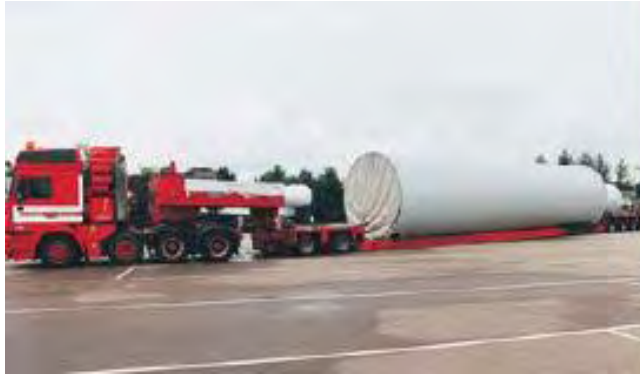
Plate 3: 20 m Tower Section on low-bed tri-axial Trailer (Very little ground clearance)
