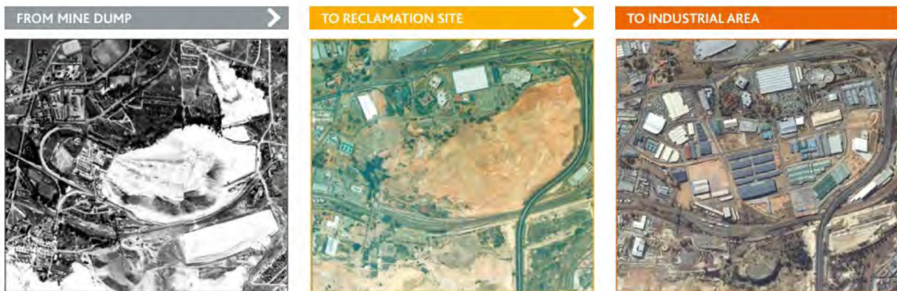
Figure 5-1: Progress of reclaiming a dump, where land was liberated for industrial development.
