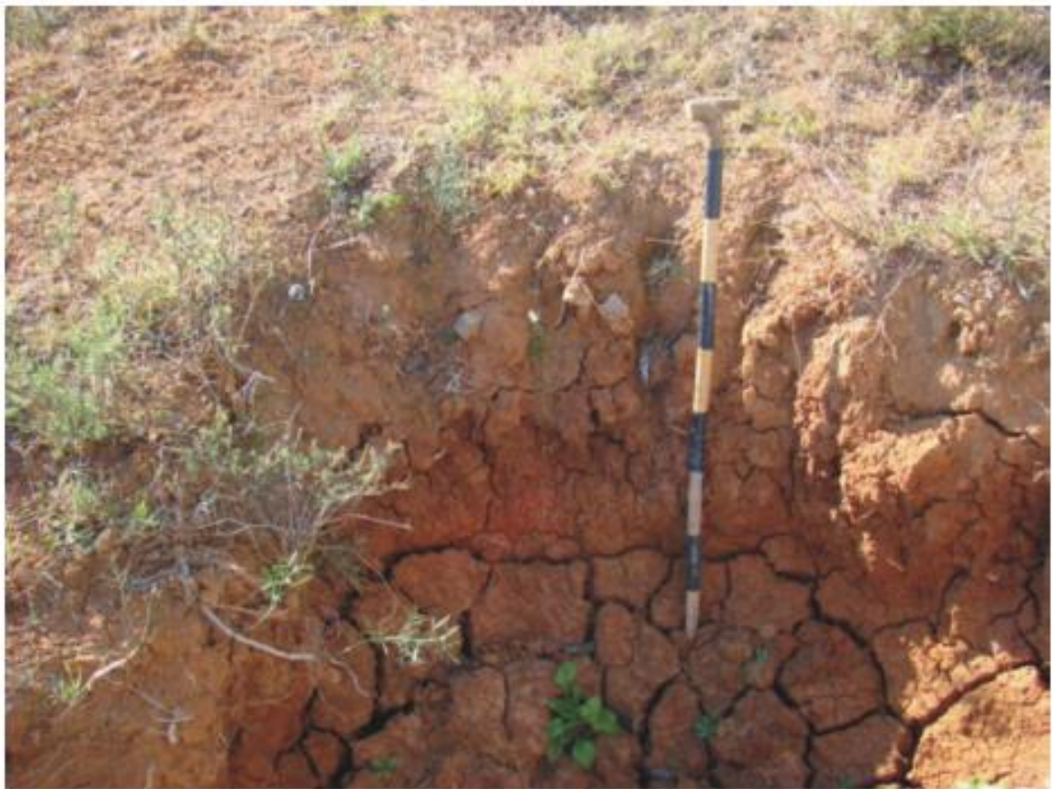
Figure 8. Test pits indicate that the site is capped by a >1m -thick mantle of Quaternary colluvium and residual soils of low palaeontological sensitivity.
