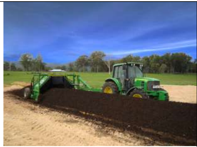
Figure 2.3 Example of a compost turner
